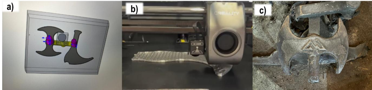
Figure 3. Steps in the casting process: a) Setup used in the SolidCast simulation, b) 3D-printed model, c) axe blade in as-cast condition.
