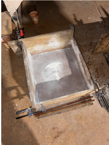
Fig. 5: Sand mold of Ax
