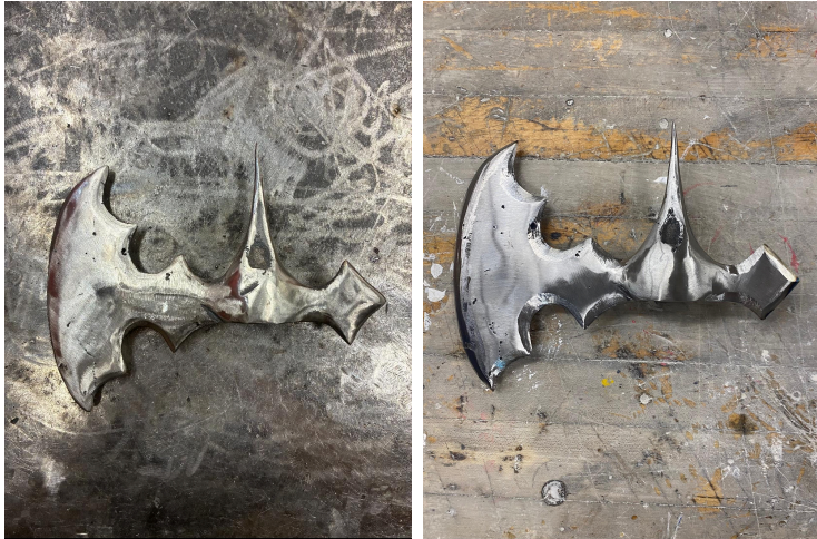
Figure 13: Axe head after initial grinding (left)
