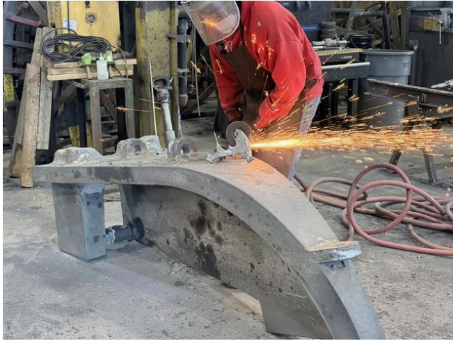
Fig. 9: Gating and riser removal (Left)
