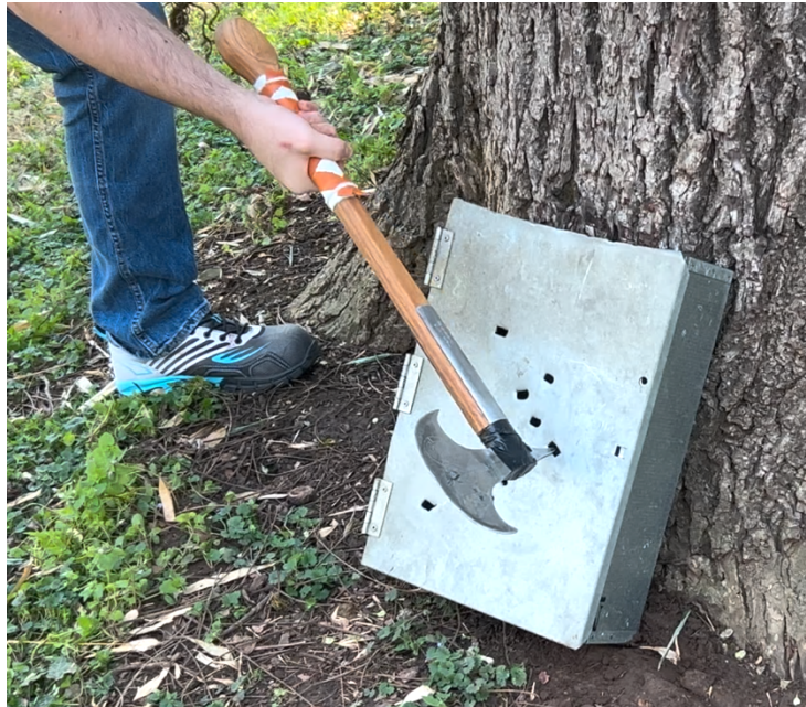
Fig. A15 Impact testing of back spike against steel plate electrical box
