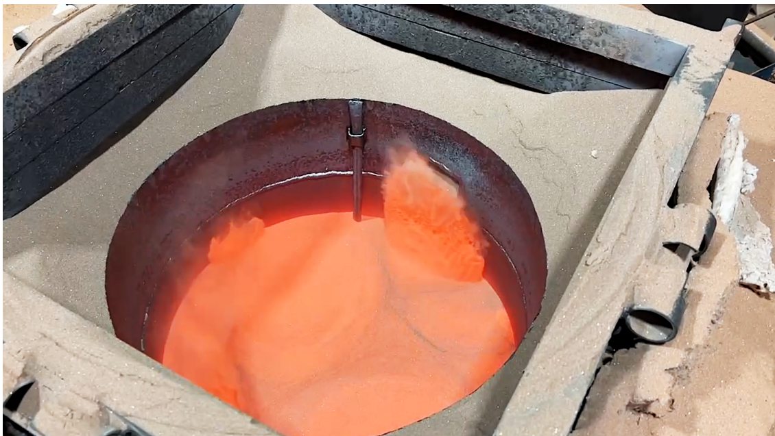
Fig. A13 Fluidized alumina oxide heat treatment furnace
