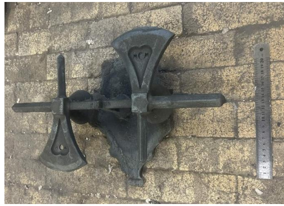
Figure 2. Casting process: (a) S&T foundry casting 3D printing molds with axes, and (b) final cast axes after breaking the sand mold.
