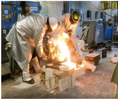
Figure 2. Casting process: (a) S&T foundry casting 3D printing molds with axes, and (b) final cast axes after breaking the sand mold.
