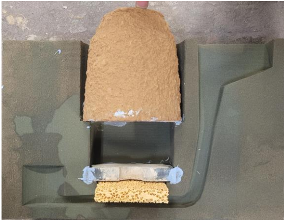
Figure 4. Image of the Y-Block casting sand mold. Note the filter, chill blocks, and riser sleeve
