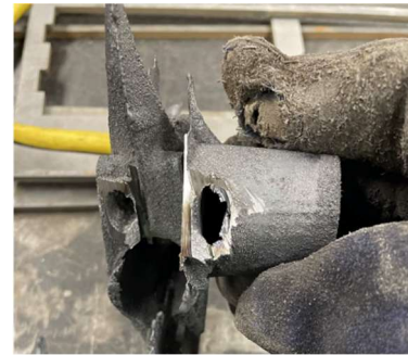
Figure 10a. Shrinkage Defect in Earlier Design.
