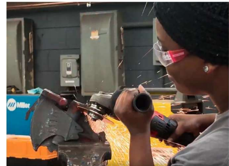
Figure 8. Engineering Student Grinding Gating Off.
