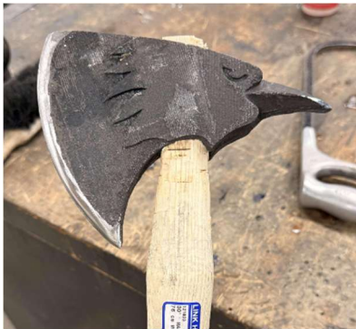
Figure 12. First Successful Axe Head Manufactured.
