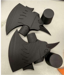
Figure 5. Half of 3D Printed Mold Cavity.
