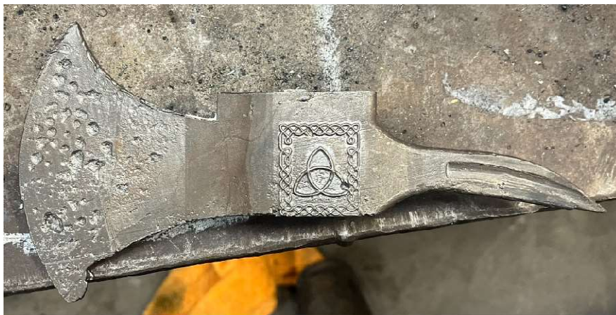
Figure 3: Initial casting with heavy surface pitting
