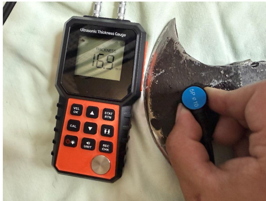
Figure 6: Using a Gauge Tester to verify Axe thickness in mm.
