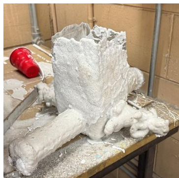
Figure 4. Investment Cast Handle Mold
