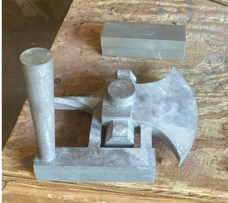
Figure 3. 3D printed models with core boxes
