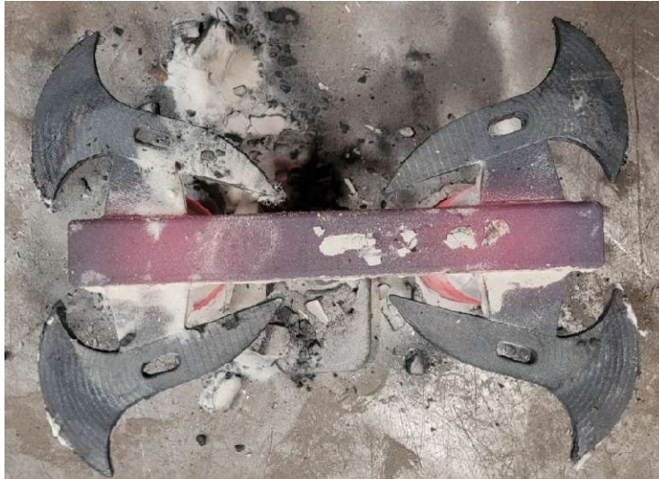
Figure 6: Solidified axe heads on gating immediately after pouring
