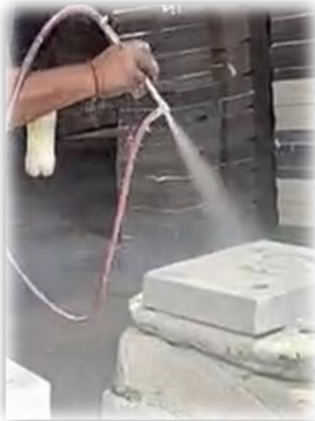
Figure 24. d) Application of refractory coating on the sand
