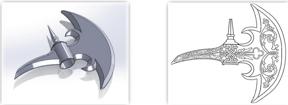
Figure 1. 3D CAD model of the horseman's axe developed in SolidWorks.
