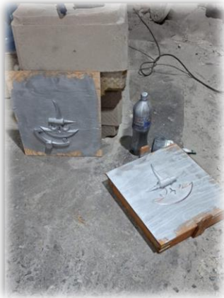
Figure 21. a) Application of the molding coating
