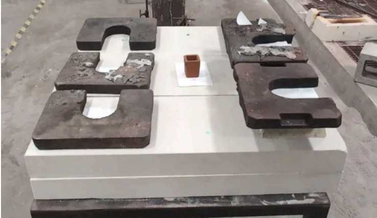
Figure 1: Assembled Molds Before Pouring.
