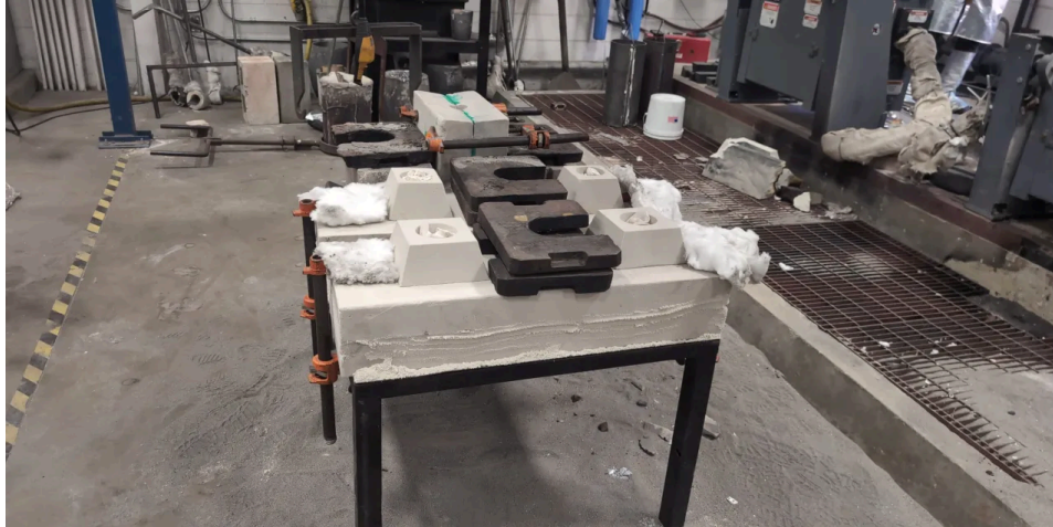
Figure 5: Assembled Molds Before Pouring.
