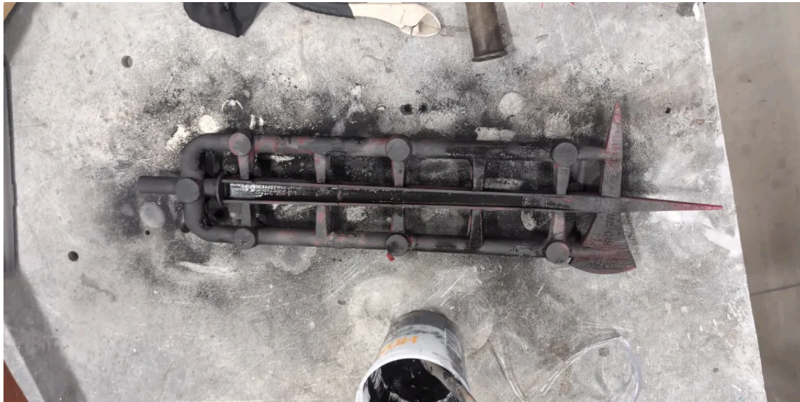
Figure 4: Prepared Loose Piece Pattern.
