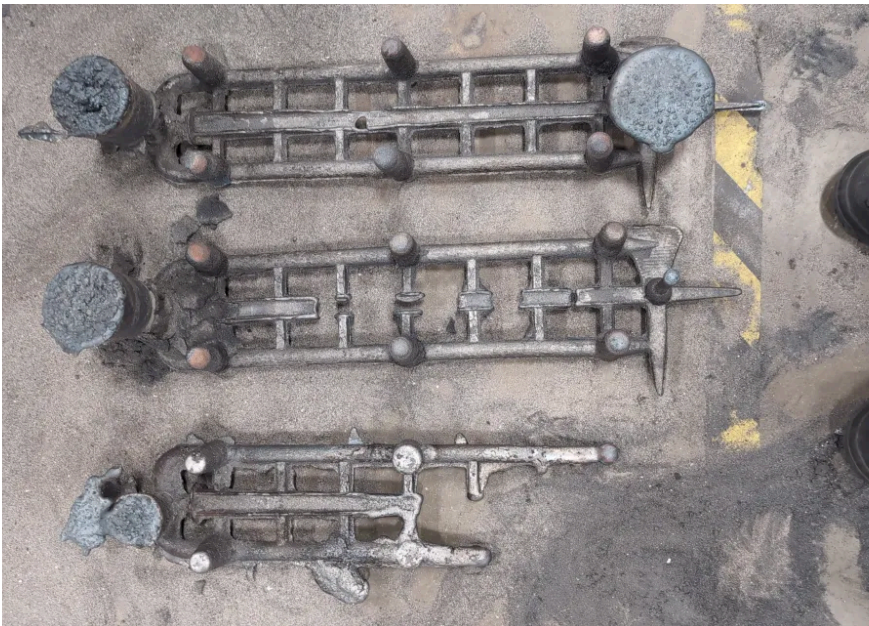
Figure 2: Castings with Defects.
