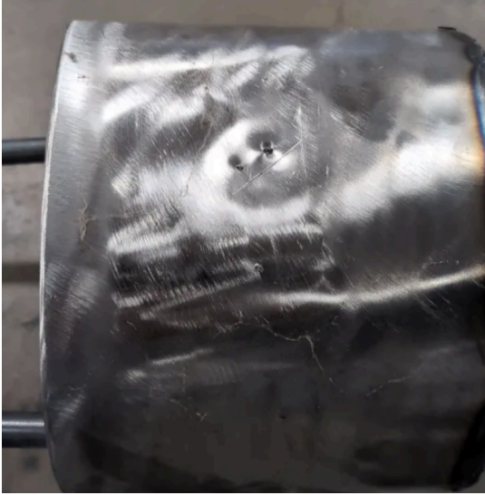
Figure 8: Plate Punctured by Axe
