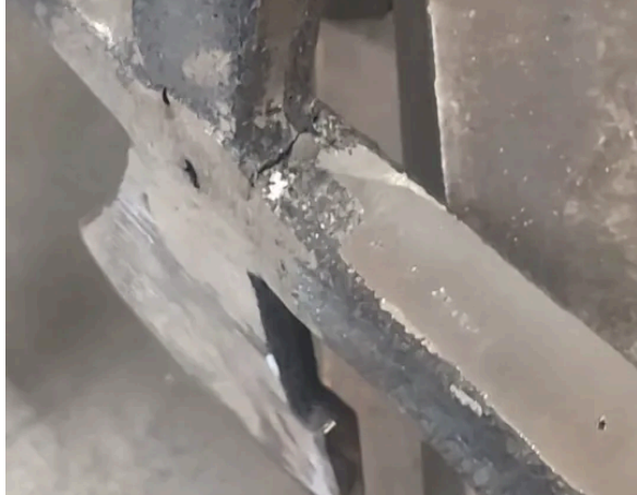
Figure 3: Hot Tear Detail.
