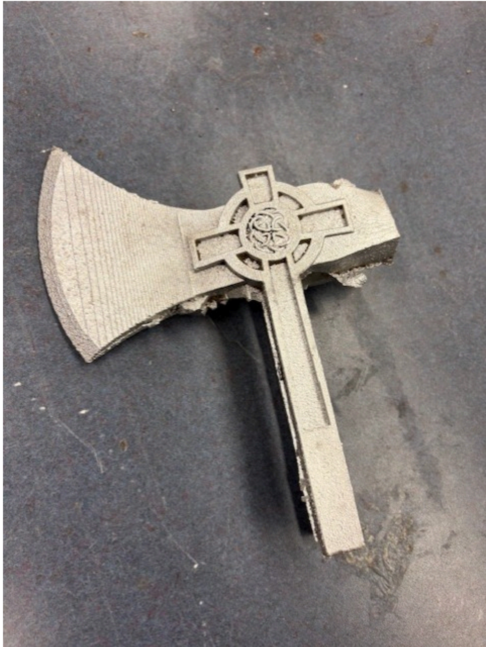
Figure 6: Aluminum test cast to verify pattern board
