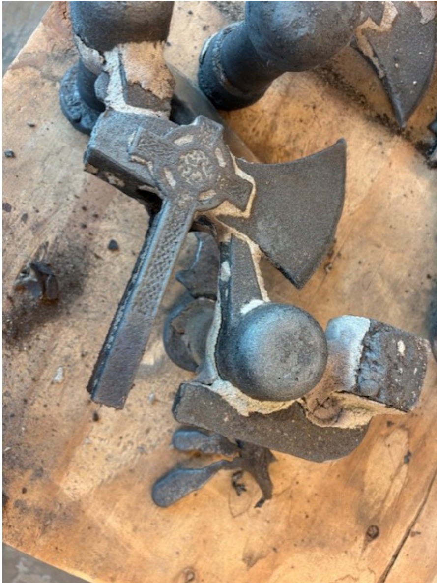
Figure 7: Successful steel pour cast on sprue
