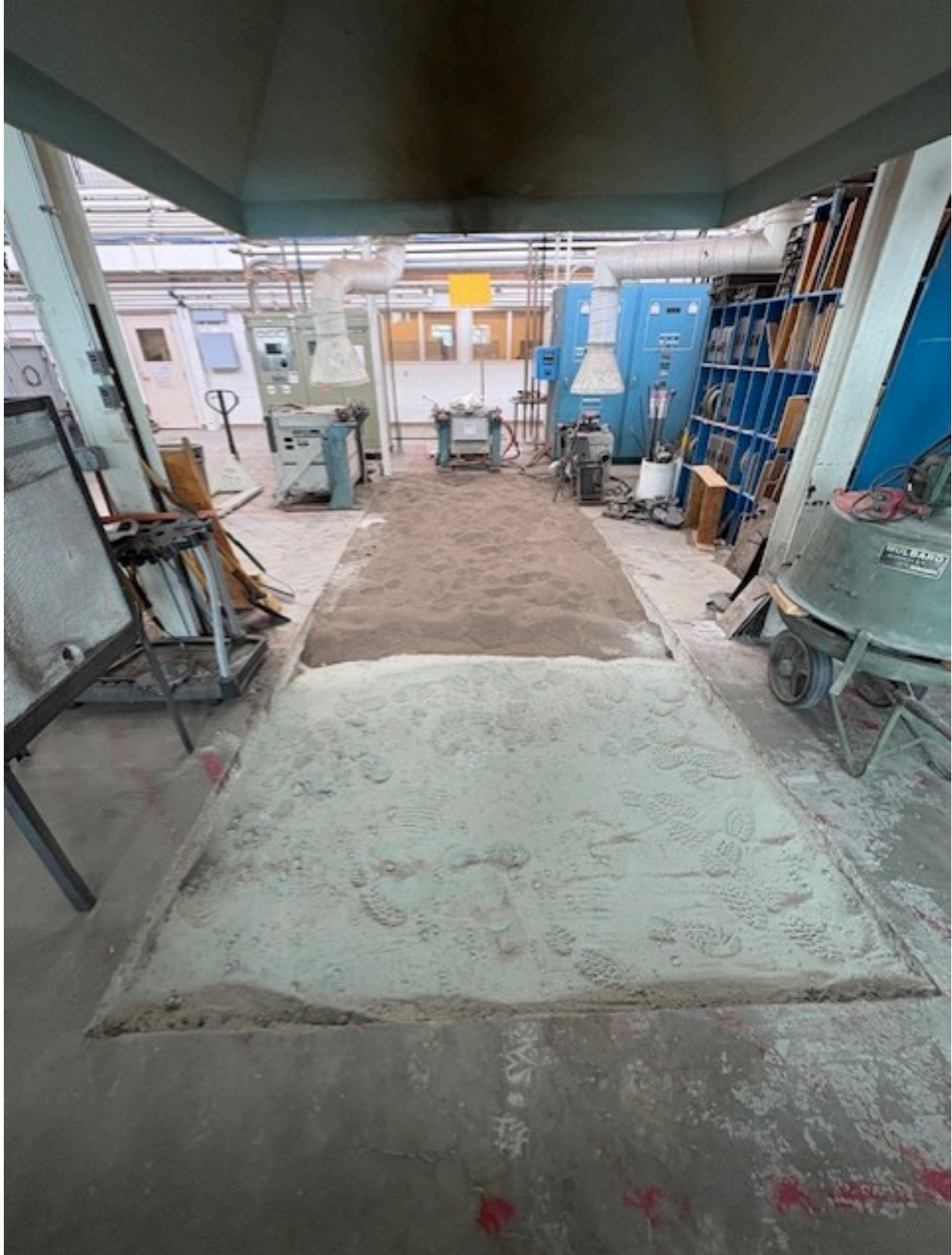
Figure 4: Old vs. new green sand
