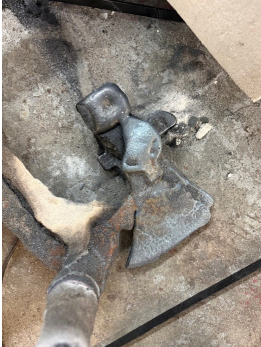
Figure 3: Failed prototype casting
