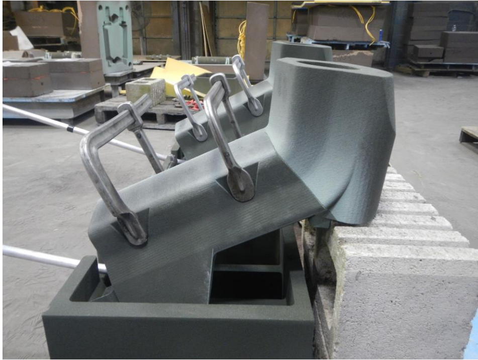
Figure 4: Assembled molds – side view
