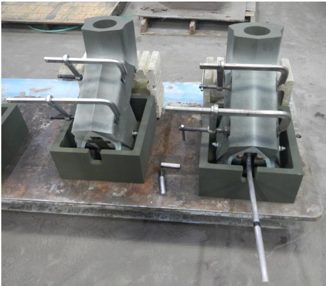
Figure 3: Assembled molds - front view
