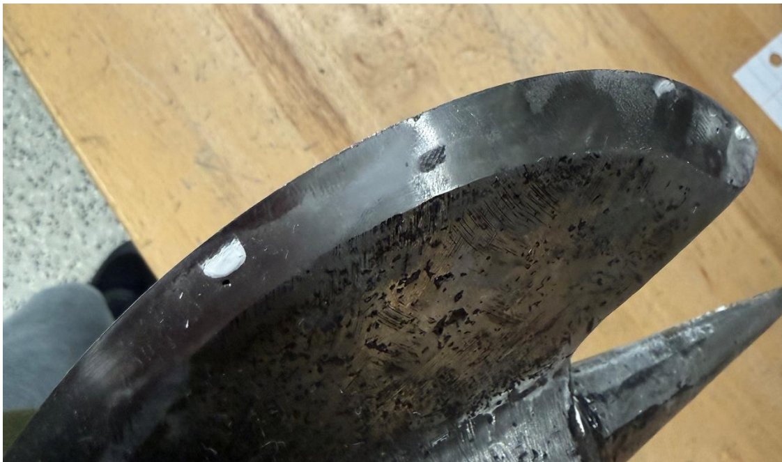
Figure 36. The second axe's blade after destructive testing, which showed slight dulling and rollover.
