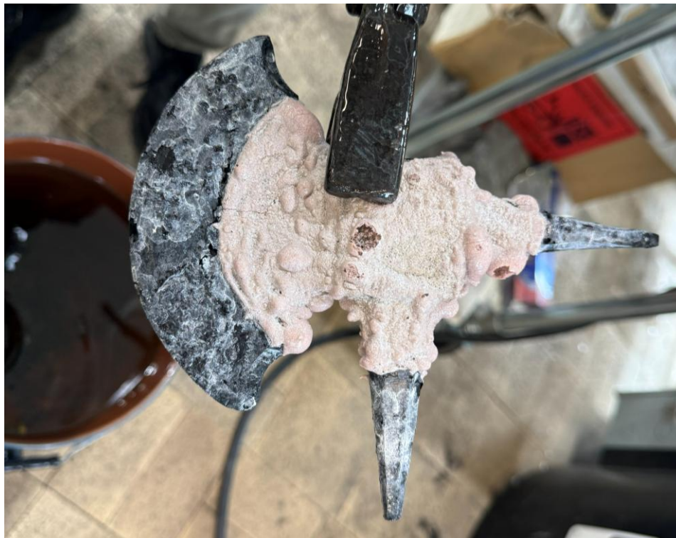
Figure 17. The refractory coating on the just-quenched axe head.
