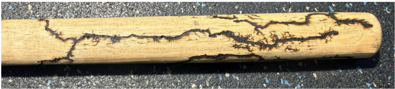
Figure 15. The Lichtenberg figures that were burned into the handle of the axe.
