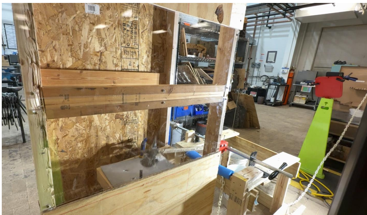
Figure 34. The testing rig chopping an 18-gauge steel plate.
