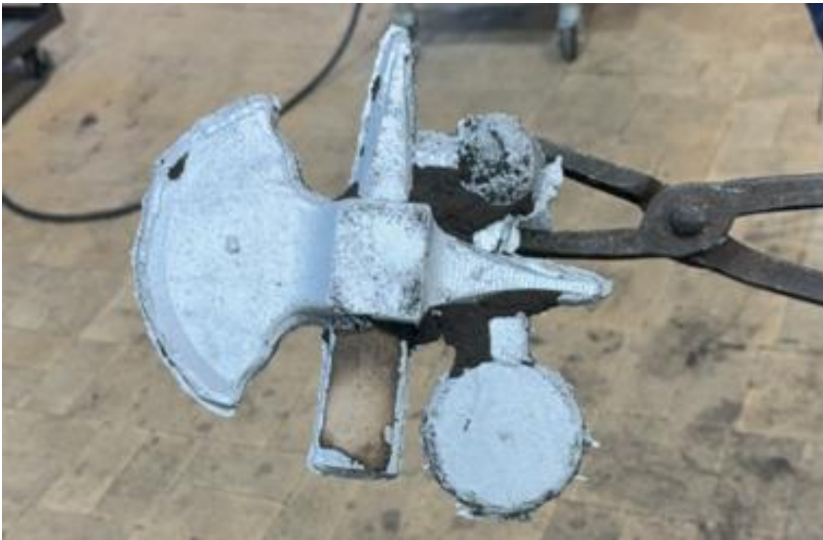
Figure 23. An aluminum pour of the final gating iteration before degating and removal of the core sand.
