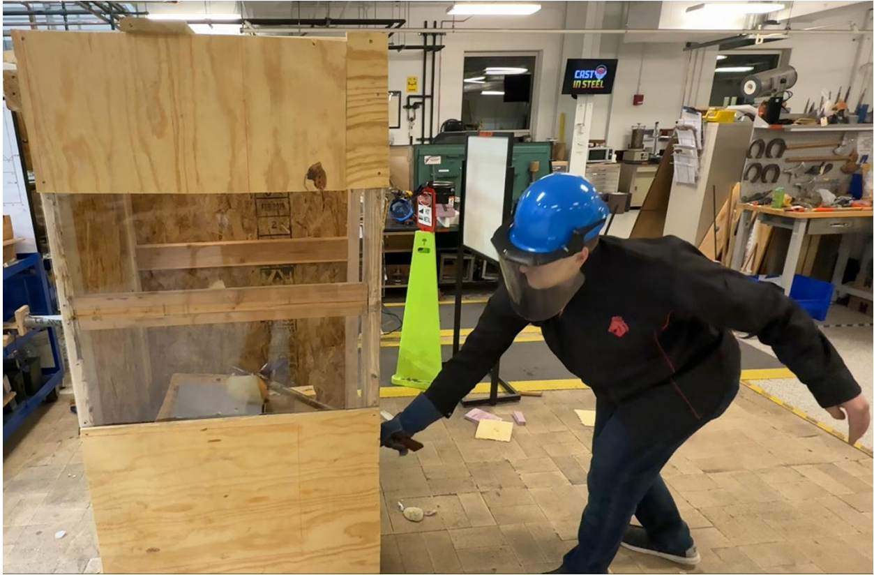
Figure 35. Hand testing the axe against the 18-gauge steel plate.
