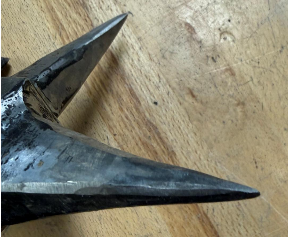
Figure 37. The second axe's pick after destructive testing, which showed no damage.
