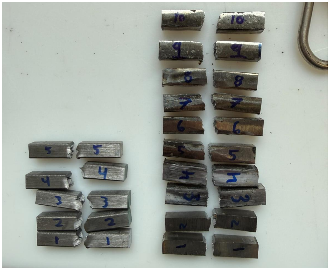
Figure 26. The Charpy impact test specimens, with “true” 4140 on the left and cast 4140 on the right.
