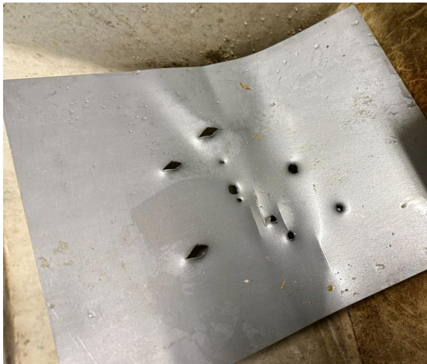
Figure 38. The 18-gauge steel plate after destructive testing.
