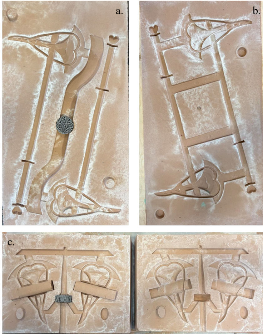
Figure 8. Finished drag (a) and cope (b) molds of handled axe, along with mold for handle-less axe (c) before casting.
