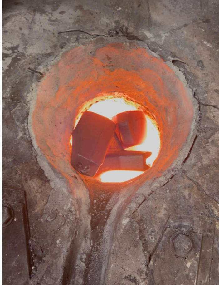
Figure 9. 50 lbs induction furnace used for casting.
