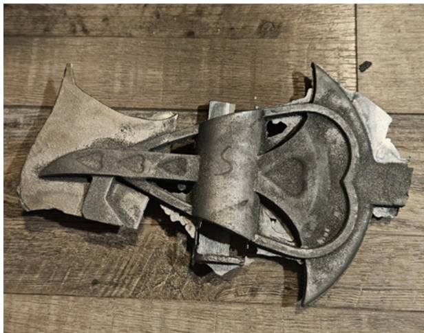
Figure 12. Example of handle-less ax before and after the fettling process.
