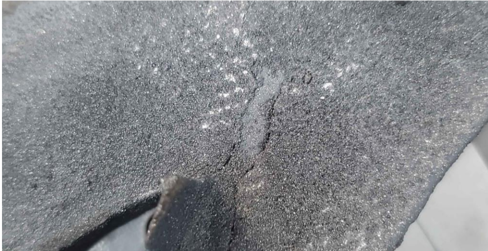
Figure 9 A cold shut on the face of the axe blade.
