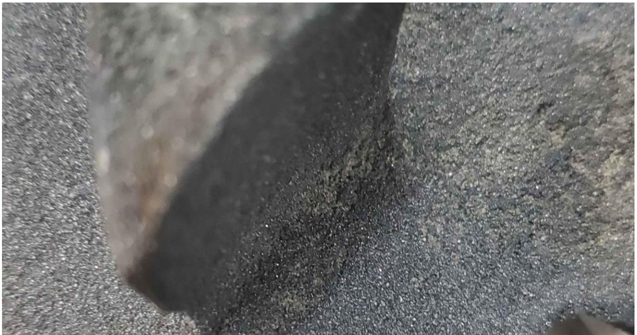
Figure 8 Sand penetration near axe blade cut-out.
