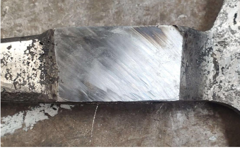
Figure 11 A cross section of the axe eye, cut to reduce weight on the axe.
