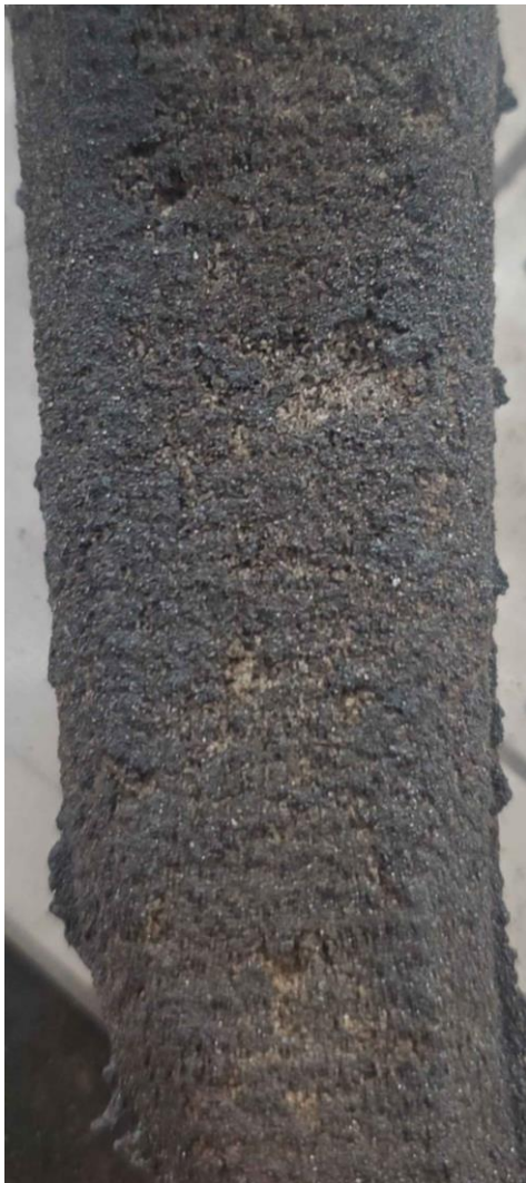
Figure 10 Sand penetration on axe spike.
