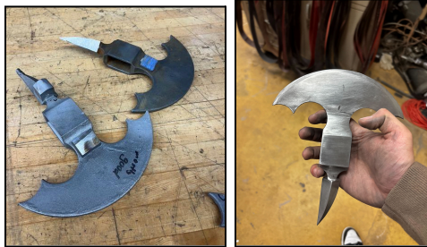
Figure 11. Photos of the axe head. Left: As-Cast with the sprues removed. Right: Axe after post-processing.
