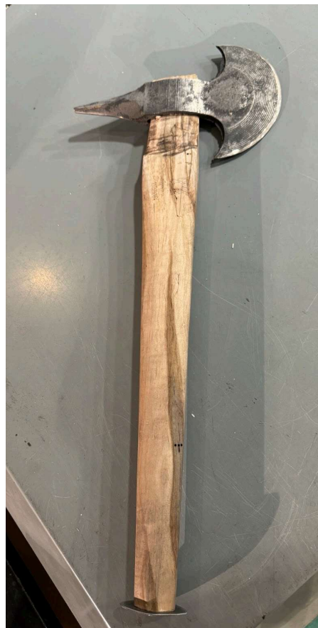
Fig F.4: Finished Trial Axe With Processed Axe Head and Finished Handle; After Testing With Broken Spike Tip
