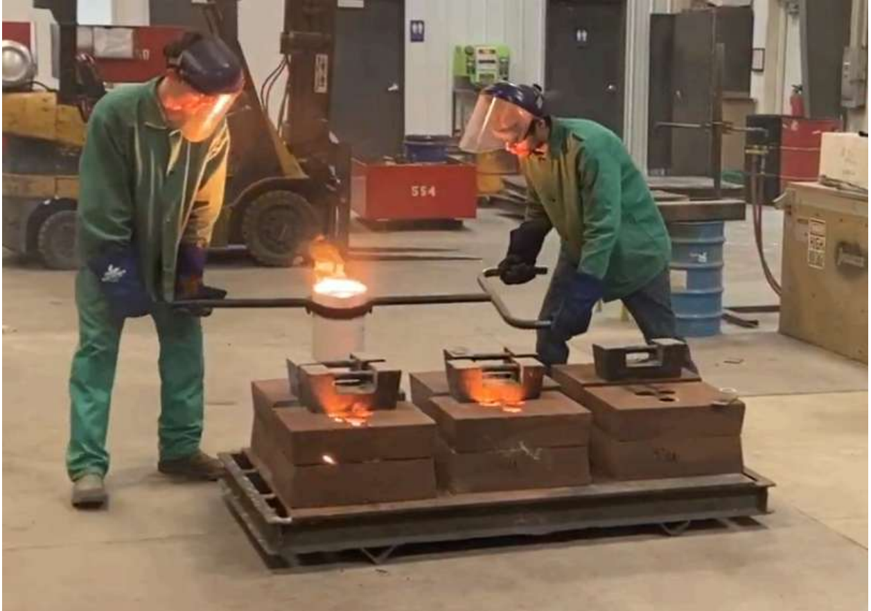
Fig C.3: Pouring at Fisher
