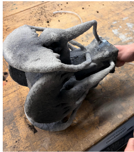
Figure 7. Burn-out and washed-out mold waiting to be pre-heated
