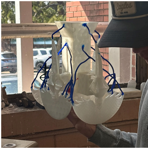
Figure 6. Assembled 3-D mold and attached vents, waiting to be poured
