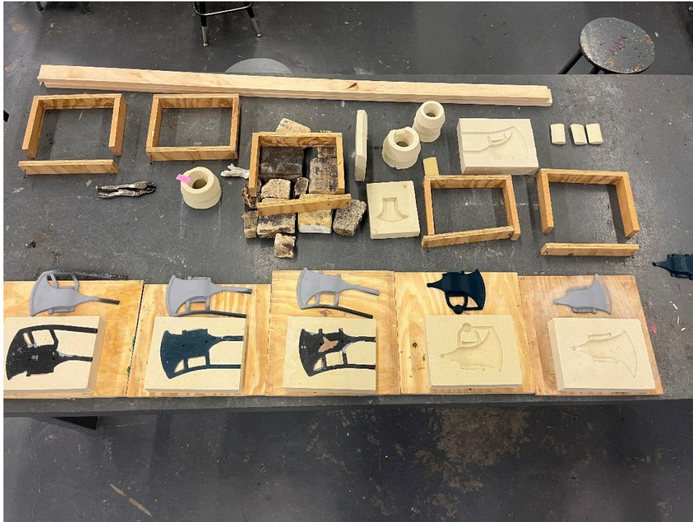
Figure 2. Five different gating designs were redundancies to ensure at least 2 would properly fill.
