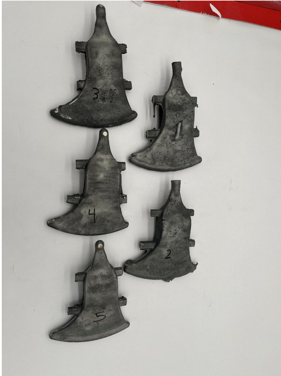
Figure 7) Axe mold box after the pour and axes after removing gating system.
