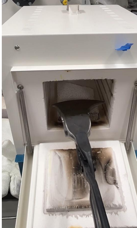
Figure 8) Insulated furnace used for annealing, quenching, and tempering the blade.
