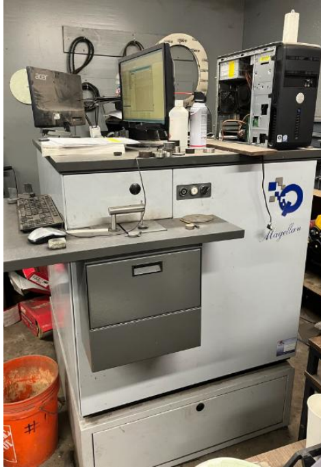
Figure 6) Optical emission spectrometer used to determine composition of a sample of the molten steel alloy prior to casting.
