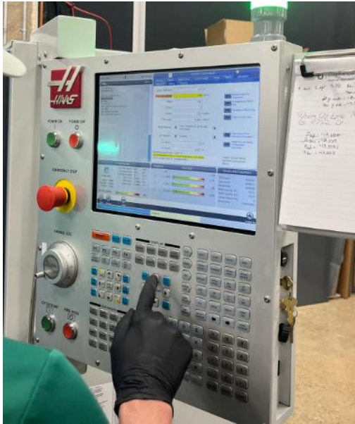
HAAS CNC machine used for subtractive machining of the axe.
