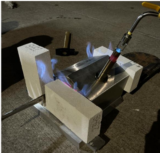
Furnace used to heat the steel for forging and melt bronze for casting
