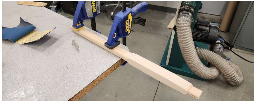
Figure 9: The full handle after machining and finishing
