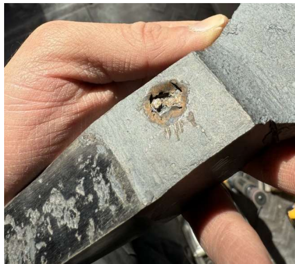
Figure 8: Large Sand inclusion uncovered from material loss due to scaling during forge welding
