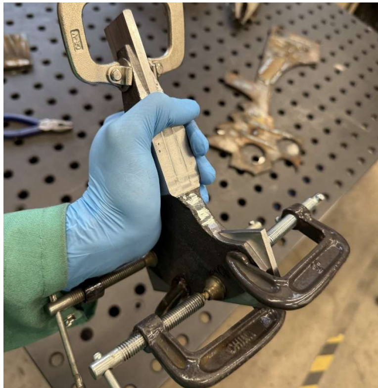
Figure 6: One of the axe heads being clamped and prepared for MIG welding
