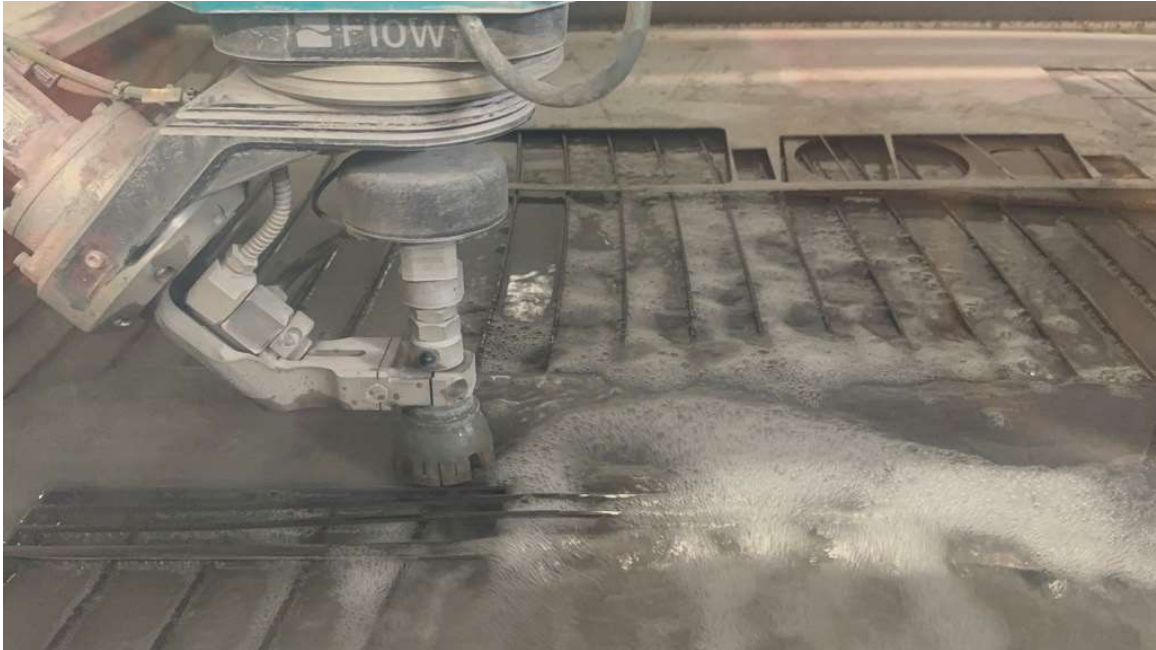
Figure 23. Water jetting langets and belt loop
