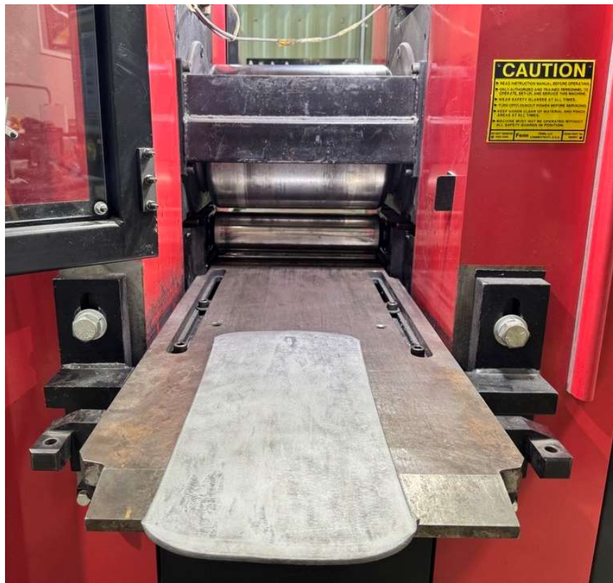
Figure 20. Hot rolled ingot prior to cold rolling
