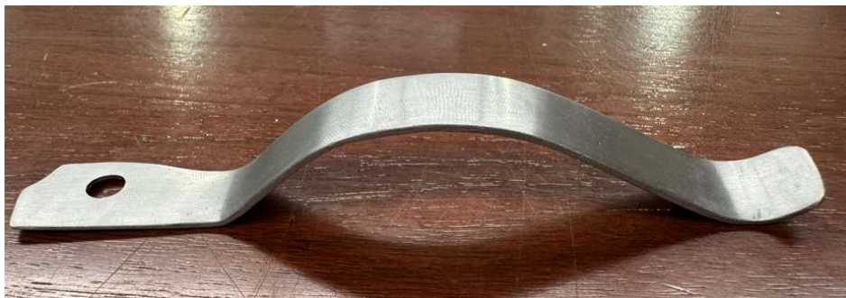
Figure 25. Forged belt loop final shape
