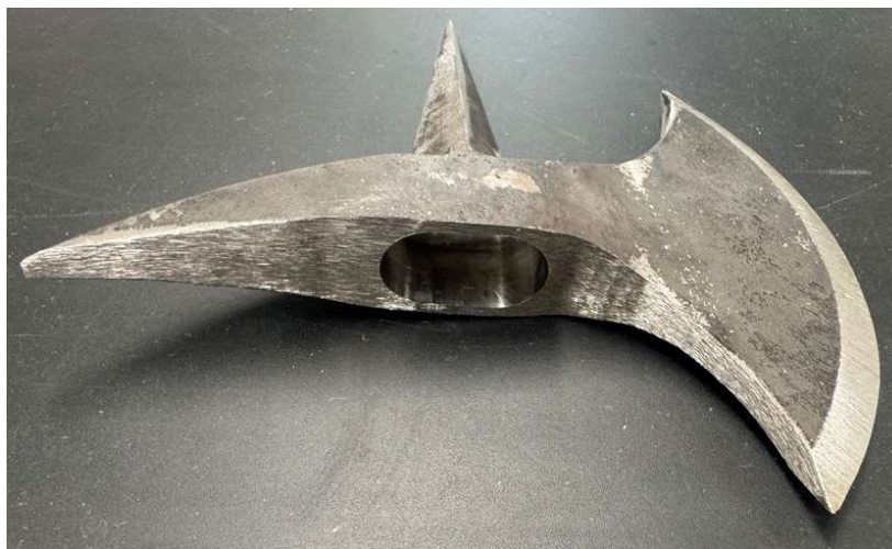
Figure 17. Drilled eye hole in bottom of axe
