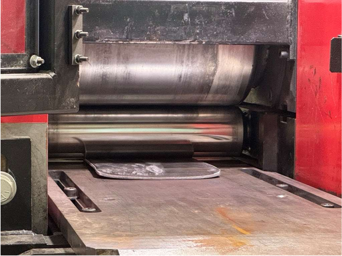
Figure 21. Cold rolling process
