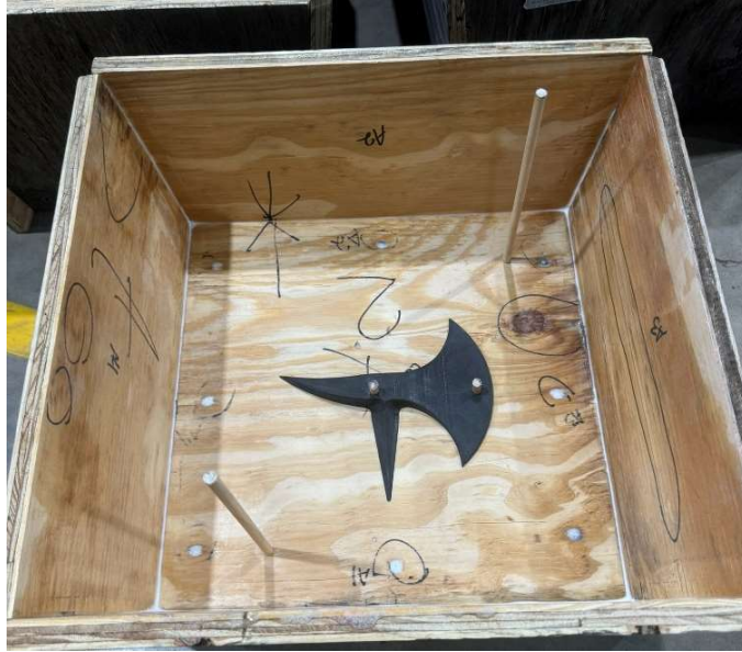
Figure 15. Mold boxes built for sand casting
