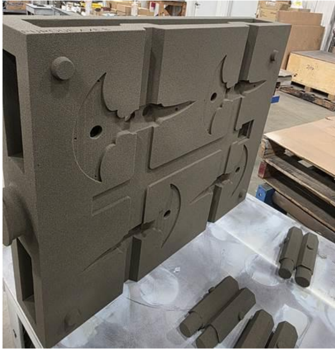
Figure 3: Binder Jet Sand Mold printed by KFA for Purdue.
