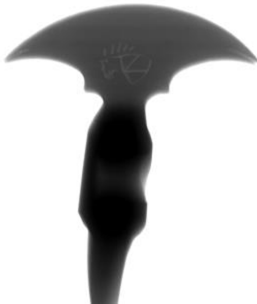
Figure 6: CT X-ray scan of a cast head provided by KFA
