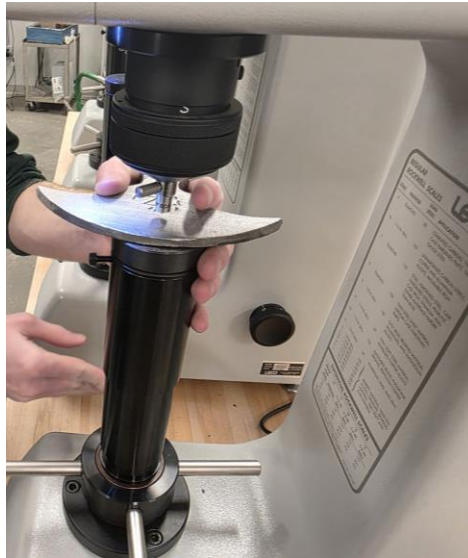
Figure 7: Using a hardness tester to test as-cast and post-heat treatment hardness.
