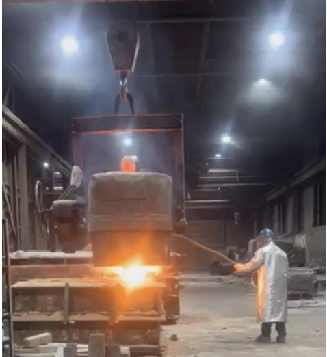
Figure [4]: Steel poured into mold
