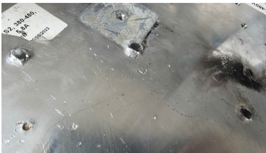
Figure 14. Results of the tests on an aluminium plate using the axe's spike.
