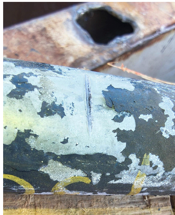
Figure 16. Cutting test results on a CF3M steel pipe.
