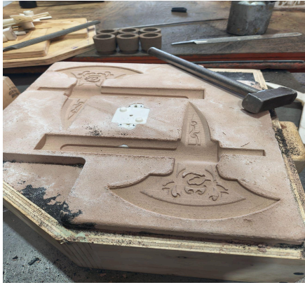
Figure 7. Half of a completed double mold after removal of the polymer patterns.
