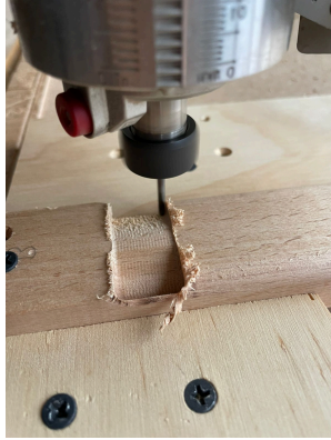
Figure 10. CNC machining process beginning the shaping of the wooden handle.
