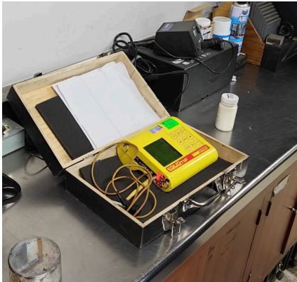
Figure 13. The Equotip actually uses the Leeb rebound method (HL) to measure hardness, which it then converts electronically to Brinell (HB).
