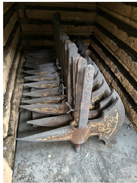
Figure 12. Axe heads undergoing annealing heat treatment.
