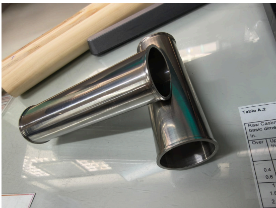
Figure 11. Machined handles prepared for abrasive carving of decorative details.
