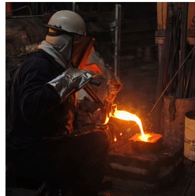
Figure 9. Melter actively pouring molten ASTM A743 Grade CA40 steel into one of the molds.
