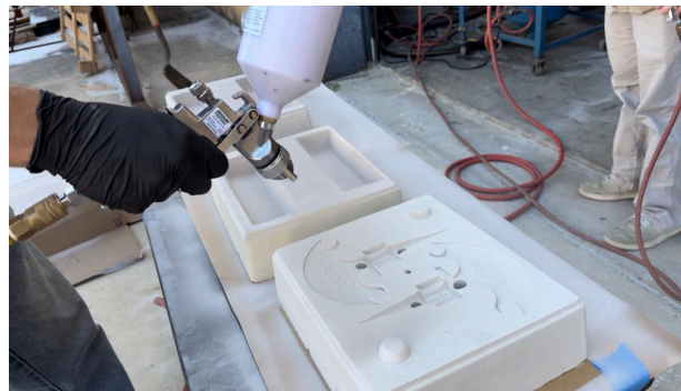
5. Spraying on mold wash.
