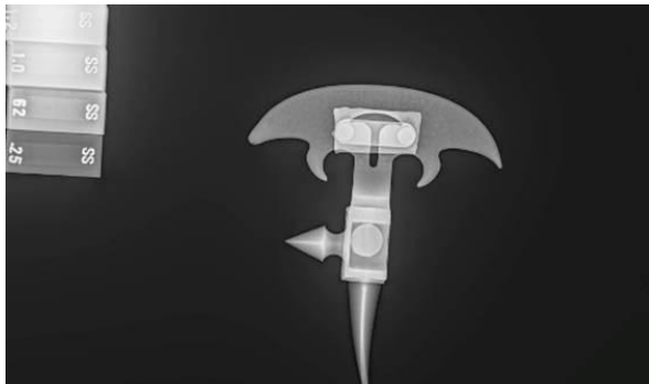
Figure 6. X-ray radiograph used to evaluate internal defects and casting quality.
