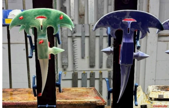
Figure 5. Tree set up for casting. The left is a PolyCast 3D print, and the right is a wax print.
