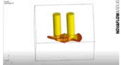
Appendix 4E Near-Final phase of pour in simulation (Design A)
