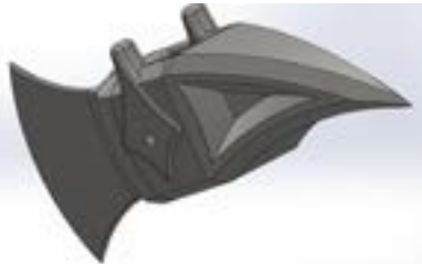
Appendix 3A reduction of initial axe design from adze to pick form
