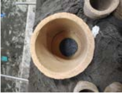
Appendix 5A Ceramic direct-pour and ceramic risers used for the casting pour with a filter in its center circumference
