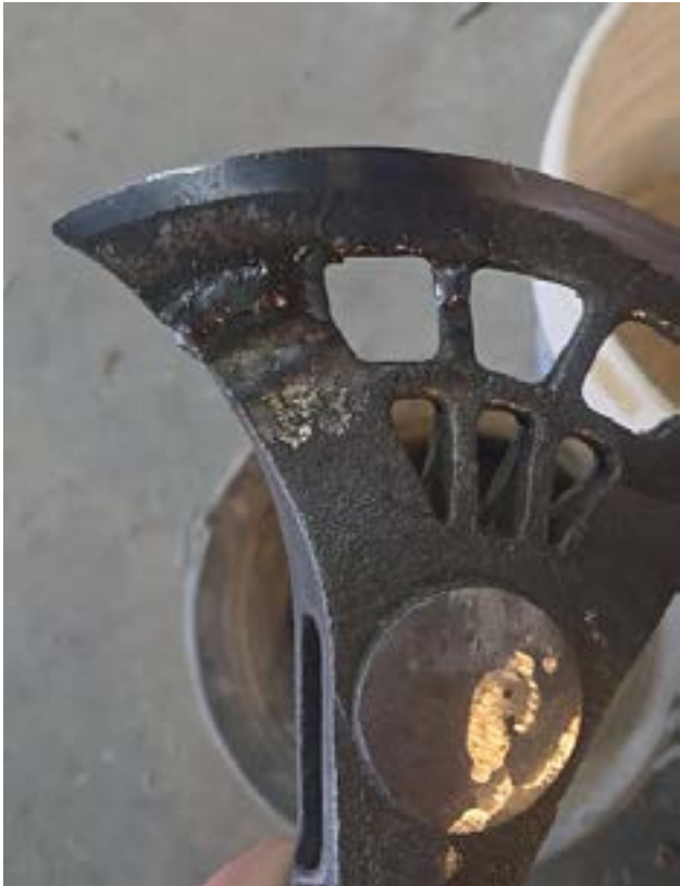
Appendix 8 Weldment of cracked Design B Axe head immediately after weldment.
