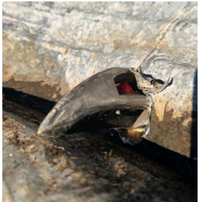
Appendix 8 Field test 1, Design B with Oak shaft tested on sheet galvanized sheet metal. (rear)
