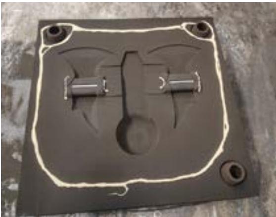
Appendix 5E Sand-cast mold of Design A
