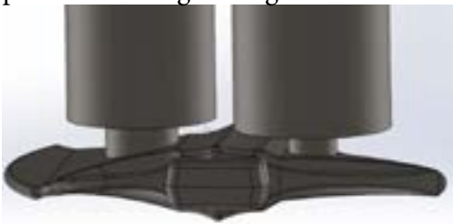
Appendix 4C Risers added to Design A prior to creating casting model
