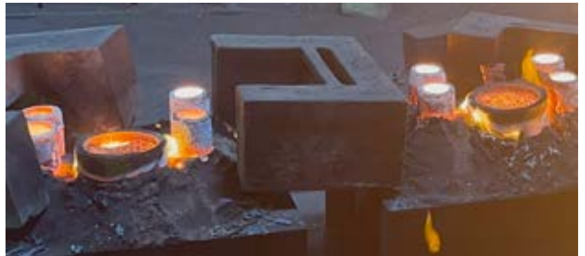
Appendix 5F (close up) Design A mold cooling after direct pour
