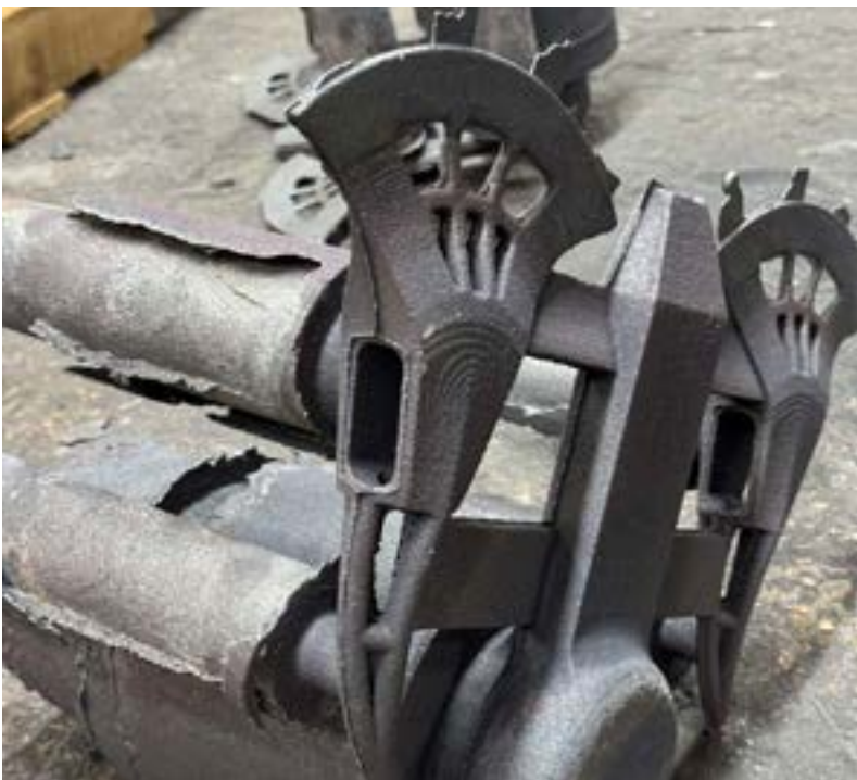
Appendix 4I uncut casting of Design B removed from sand mold
