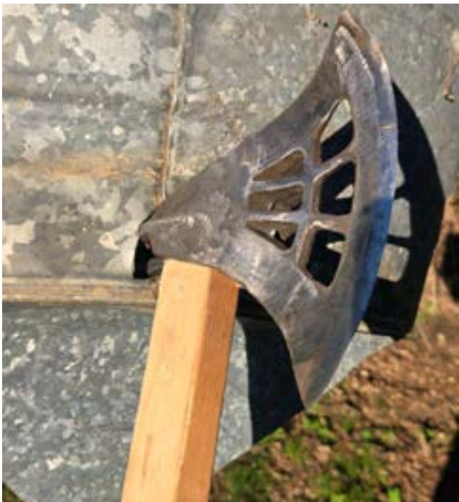
Appendix 8 Field test 1, Design B with Oak shaft tested on sheet galvanized sheet metal. (front)
