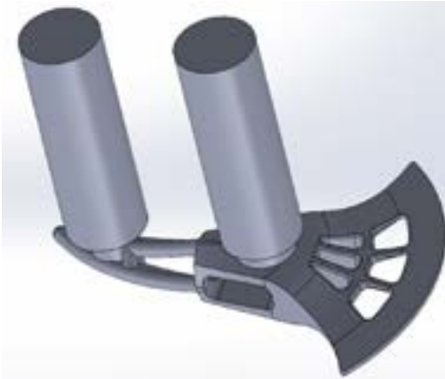
Appendix 4A Risers added to Design B prior to creating casting model
