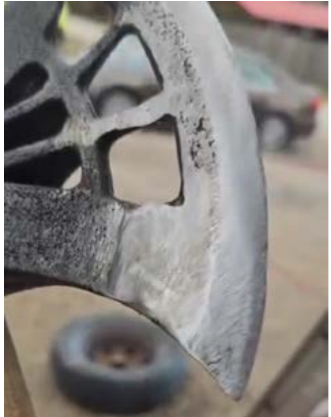
Appendix 8 Previously cracked Design B Axe head after grind and polishing.
