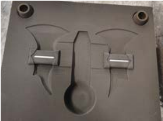
Appendix 5D Sand-cast mold of Design A
