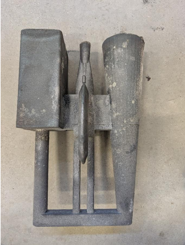
Figure 22. Raw casting from Mold 2.9.
