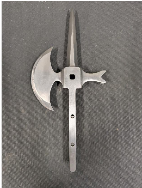
Figure 27. Axe after polishing before assembly.
