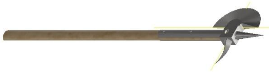
Figure 1. One of three concepts from the concept selection. This concept was rejected based upon the curved rear spike being prone to casting defects.
