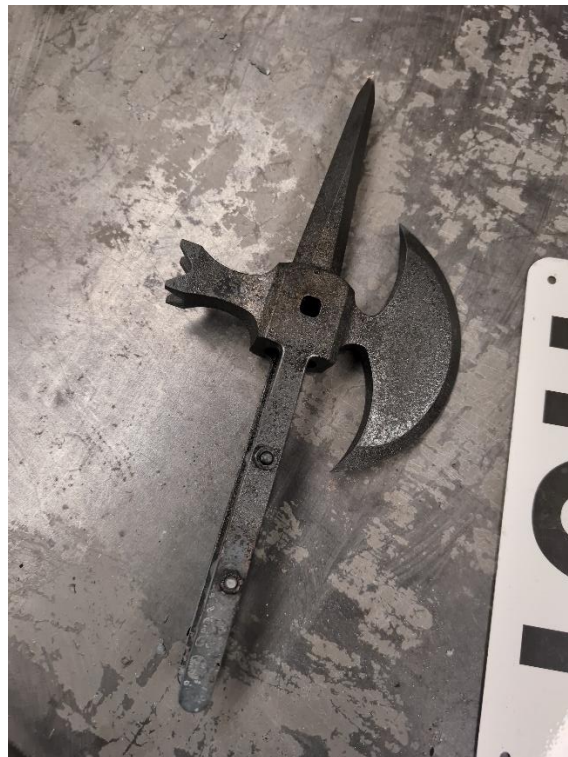
Figure 25. The machined axe immediately after quenching and tempering.
