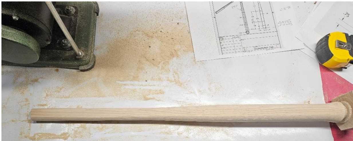
Figure 21. The haft after being shaped by the belt sander, and ready for final sanding and fit.
