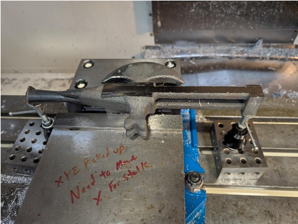
Figure 23. Casting that had gating removed and a flat surface established for datum surface creation.
