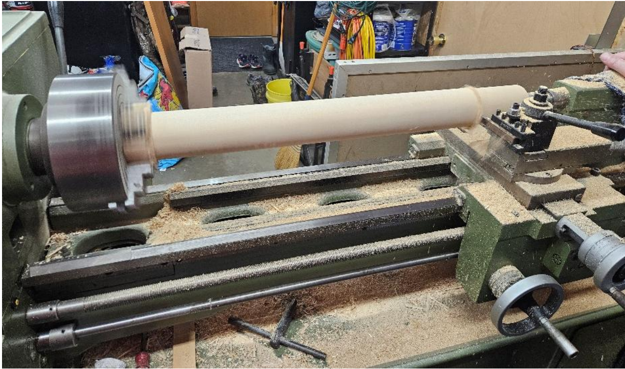
Figure 20. The haft being turned on a lathe.
