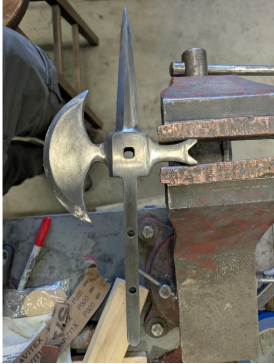
Figure 26. Axe with ground edges in the middle of polishing.
