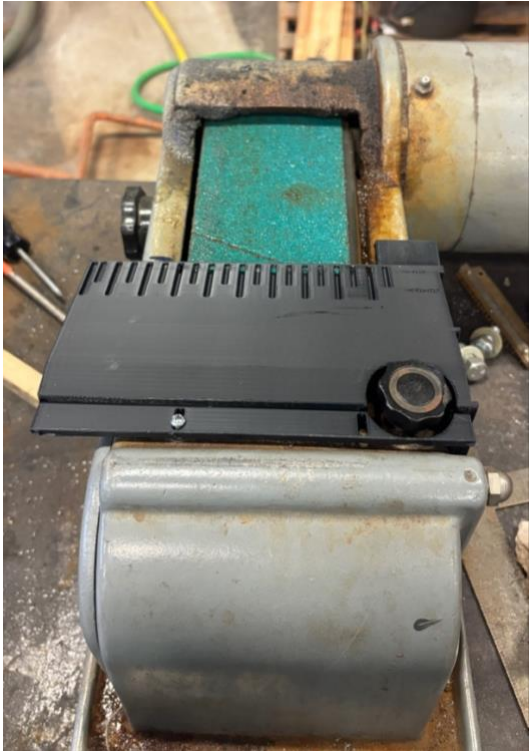
Figure 20: Failed jig with motor interference
