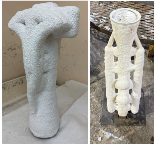
Figure G4: Ceramic Shell Mold Before Pouring
