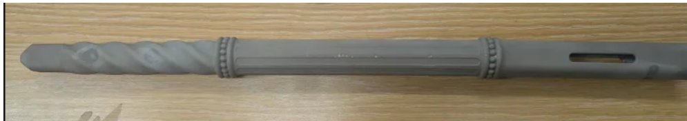
Figure G12: Finished Shaft After Heat Treatment
