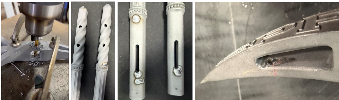
Figure G10: Post Processing (Drilling, Grinding out Defects, Before Welding, After Welding)
