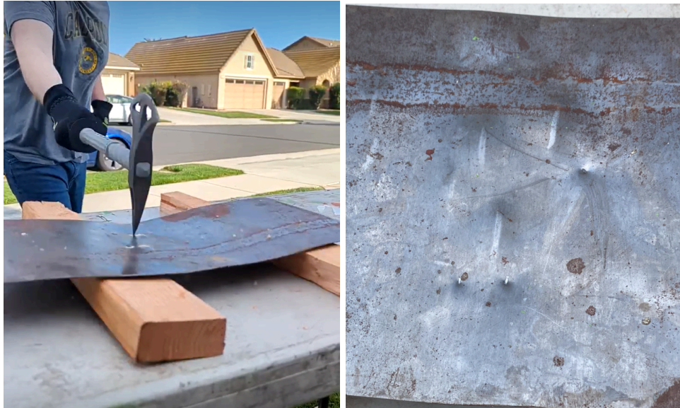
Figure 13: Back-Spike Penetration on 14-Gauge Sheet Metal
