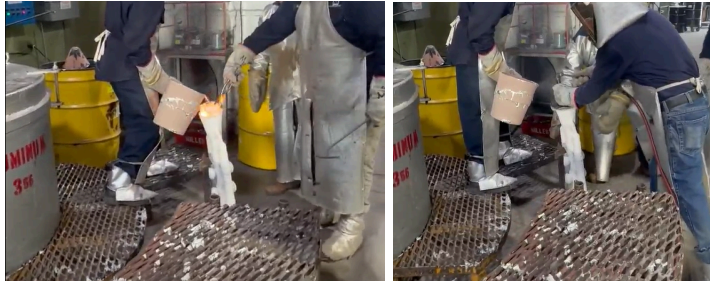
Figure G7: A356 Aluminum Metal Pouring
