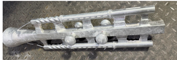
Figure G9: Raw Shaft Casting After Knockout
