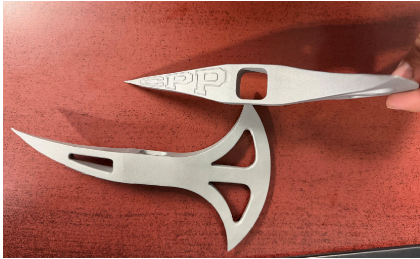
Figure G11: Finished Axe Head After Heat Treatment
