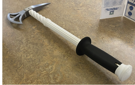
Figure G1: 3D Printed Full-Scale Prototype Assembly
