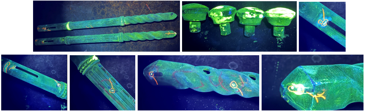
Figure E4: Aluminum Shaft Liquid Penetrant Inspection
