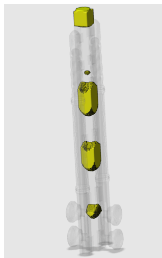
Figure F9: SolidCast Results, Axe Shaft (After Iterations)
