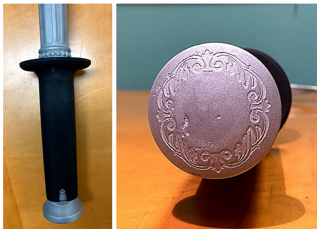
Figure H5: Detail of TPU Grip and Pommel
