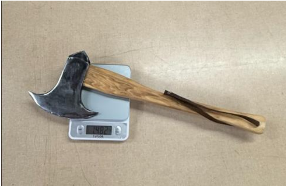
Figure G1 – Final Axe Weight at 1.482 kg
