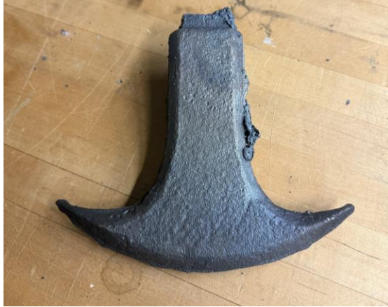
Figure D7. Post Cast - Back Spike Cut Off
