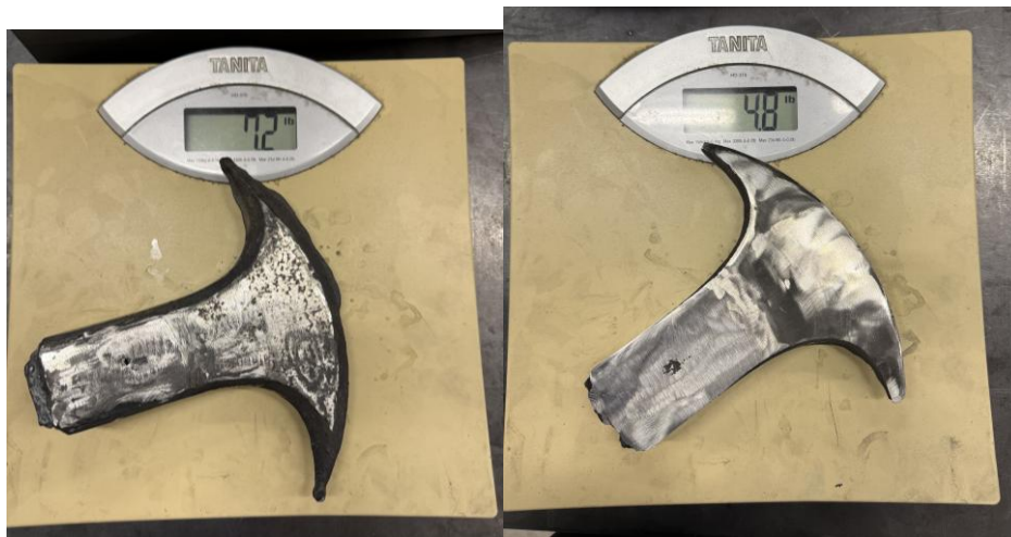
Figure E1. Machining Photos (CNC Weight Reduction)
