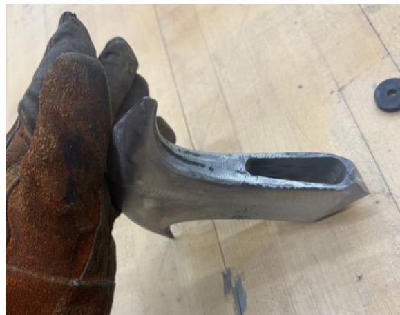
Figure E3. Machining Photos (Pocket Cut Out)
