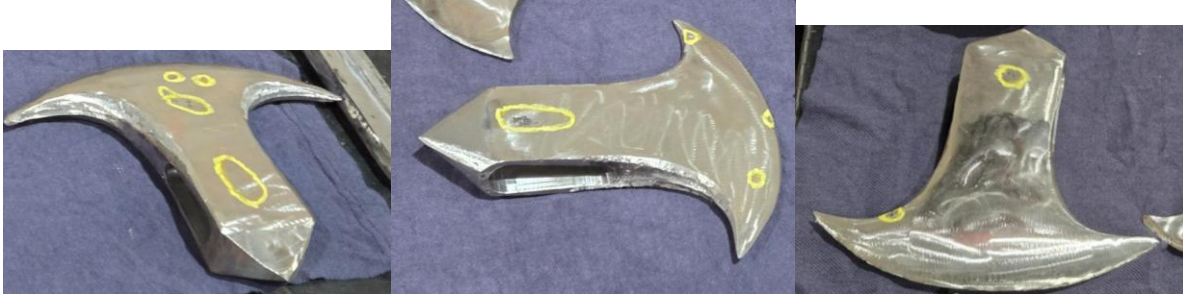
Figure F3. NDT Images (Magnetic Particle)
