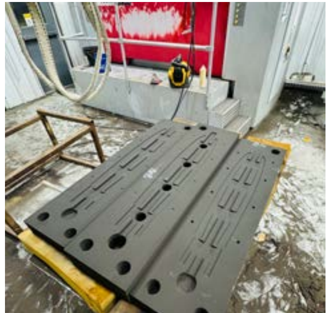
Above: Final sand-cast molds for the blade, with copes and drags laid out for visibility.
