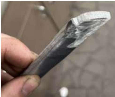
Above: The Fracture Point of the initial, carburized, and tempered blade, only a day before shipment.
