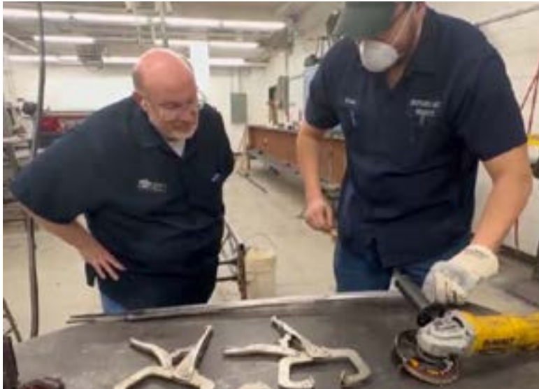
Above: Dr. Timothy Arquitt assesses and advises Juan Montoya on the grinding processes for further material removal before a series of heat treatments will begin.
