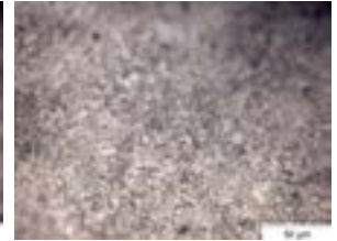
Above: OES imaging from within the fracture point of the broken sword.
