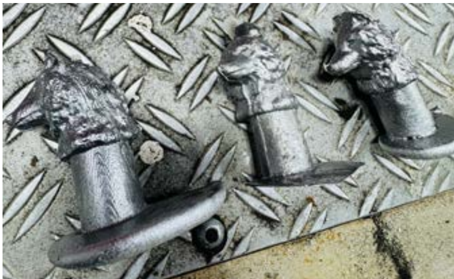
Above: Later designs cast in 319 Aluminum for use in the final sword
