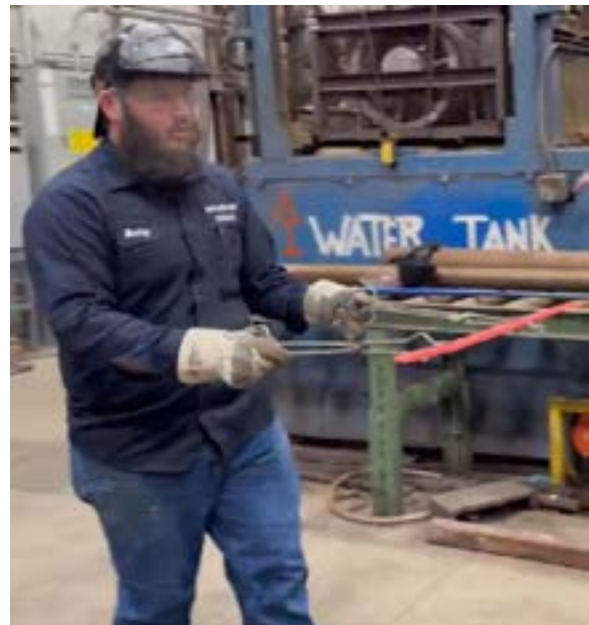
Above/Left: Henry Selig removes the swords from the normalization processing.
