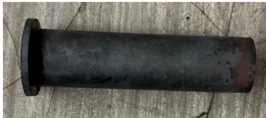
Figure 56 Quenched Jominy test bar
