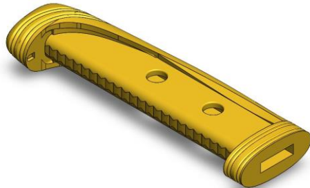
Figure 34 SolidWorks model of the handle
