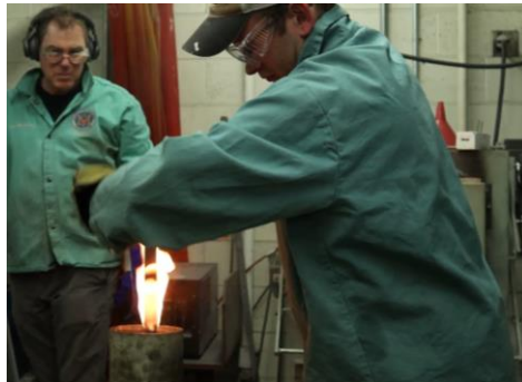
Figure 31 Sword being quenched in soybean oil
