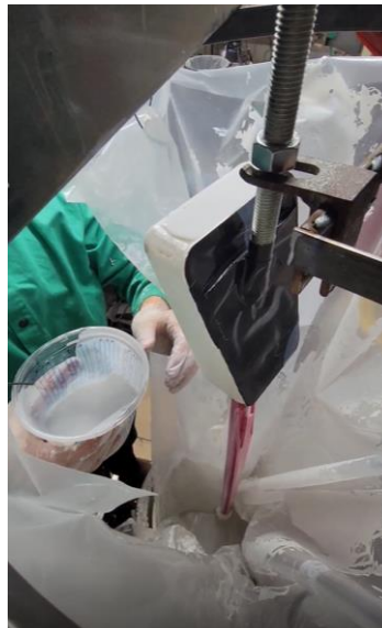
Figure 21 Applying slurry to the wax pattern
