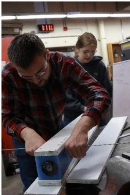
Figure 16 Separating the silicone mold
