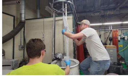
Figure 23 Applying slurry on complicated sections using a syringe
