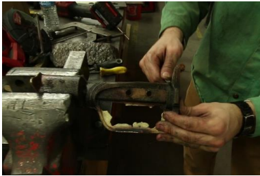
Figure 41 Filing and removing gating from the casting
