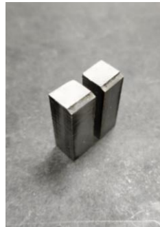
Figure 60 Charpy V-notch sample post testing
