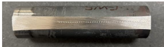
Figure 57 Jominy Bar after hardness testing
