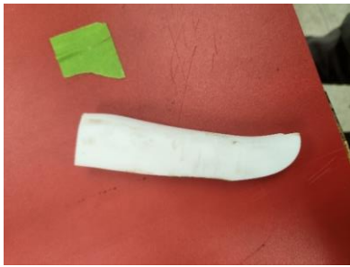
Figure 47 3D printed handle core
