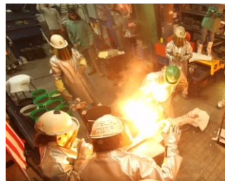
Figure 28 Modified 5160 Steel Poured
