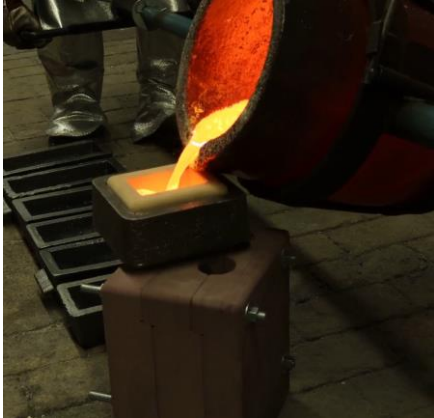
Figure 39 Pouring the C87850 Ecobross
