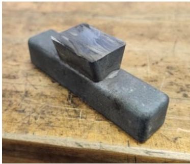
Figure 59 As cast Charpy V-Notch sample
