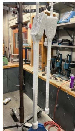
Figure 25 Final layer of "Shell" mold
