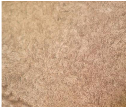
Figure 65 Quench and temper structure 1000x magnification
