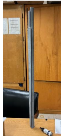
Figure 15 3D Printed resin wax pattern to be cast in silicone
