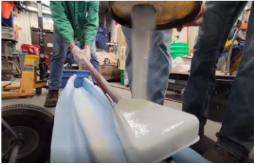
Figure 22 Shaking Zircon Sand onto the wax pattern
