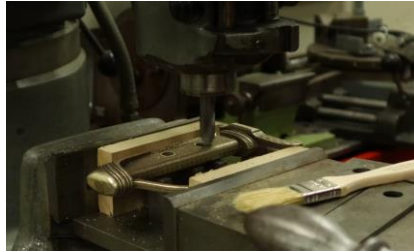
Figure 42 machining final dimensions into casting
