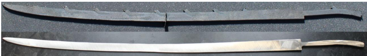
Figure 20. Blade before and after machining and finishing.
