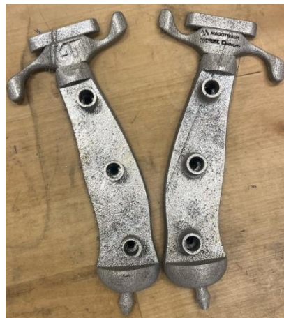
Figure 15. 3D printed scaffolding for separate-component design.
