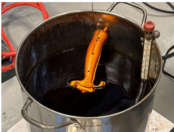
Figure 27. Anodizing of the cross guard-handle assembly.
