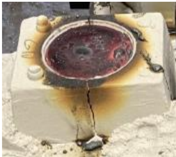
Figure .7 - Pouring cup placed on top of the sprue with core glue and no-bake sand.
