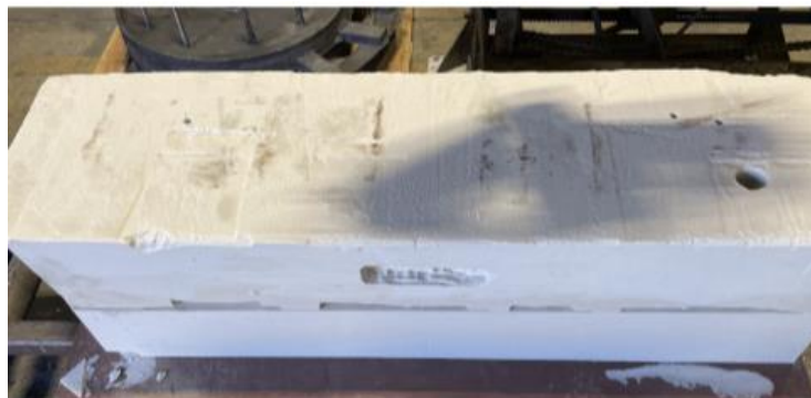
Figure .5 - Drag mold with locator pins and core mold with the sword geometry.
