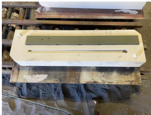
Figure .5 - Drag mold with locator pins and core mold with the sword geometry.
