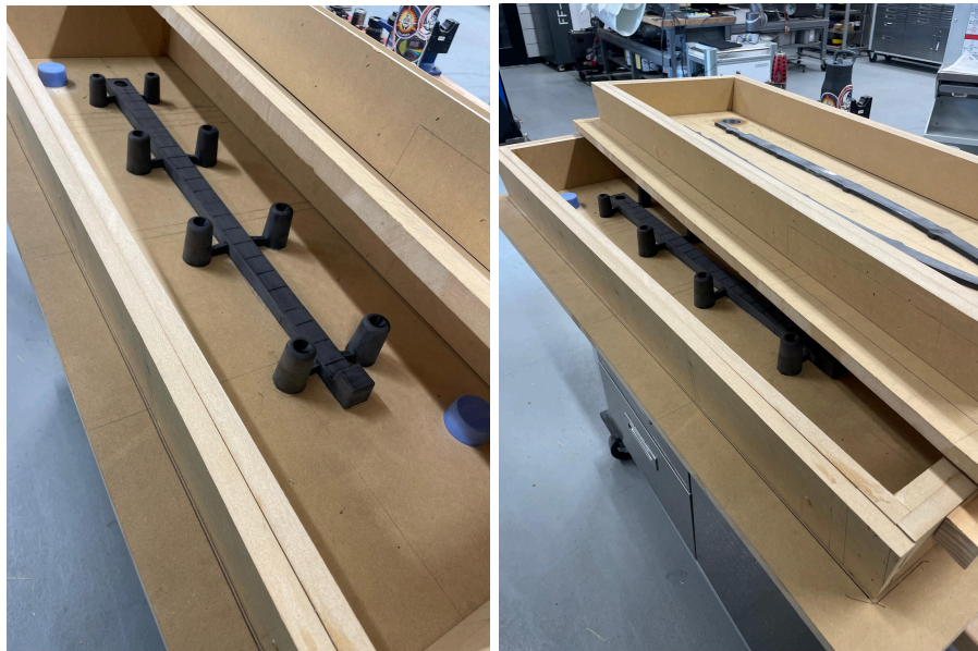
Figure 11: Left - Drag box containing gating system pattern. Right - Cope and drag boxes
