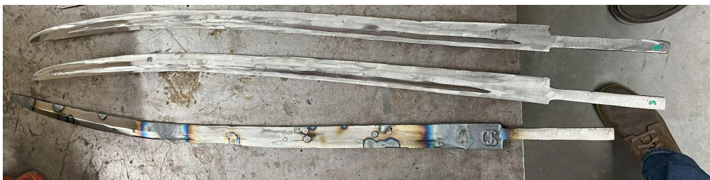
Figure 14: Blade with weld beads and finished blades.
