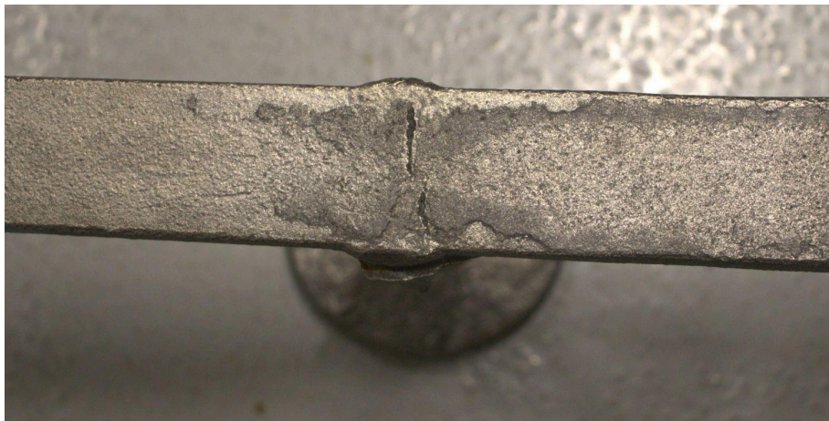
Figure 13: Un-welded hot tears
