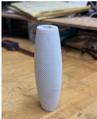
Figure 19: Final TPU 3D printed handle
