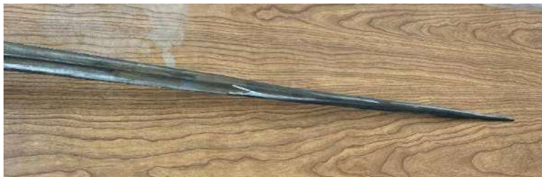
Figure 15. Sword appearance after etching with ferric chloride solution
