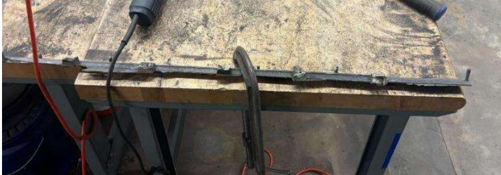
Figure 14. As-cast sword blade after removing the gating system
