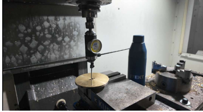
Figure 16. Cross guard preparation for the Epee made from brass alloy
