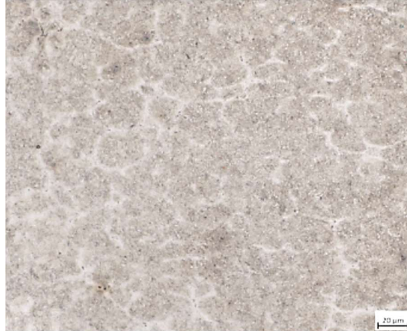
Figure 19. Microstructure of the steel after heat treatment showing presence of fine lath tempered martensite
