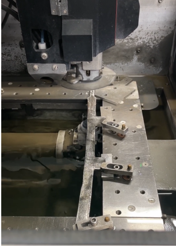
Wire EDM used to cut the sawtooth pattern into the blade using 2D CAM.
