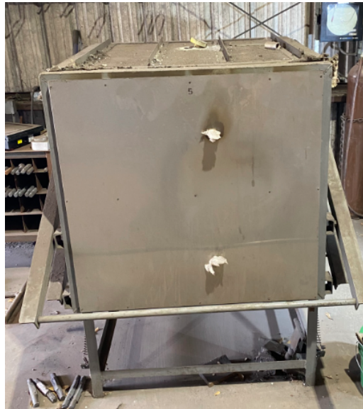
Figure 8) Insulated furnace used for annealing, quenching, and tempering the blade.
