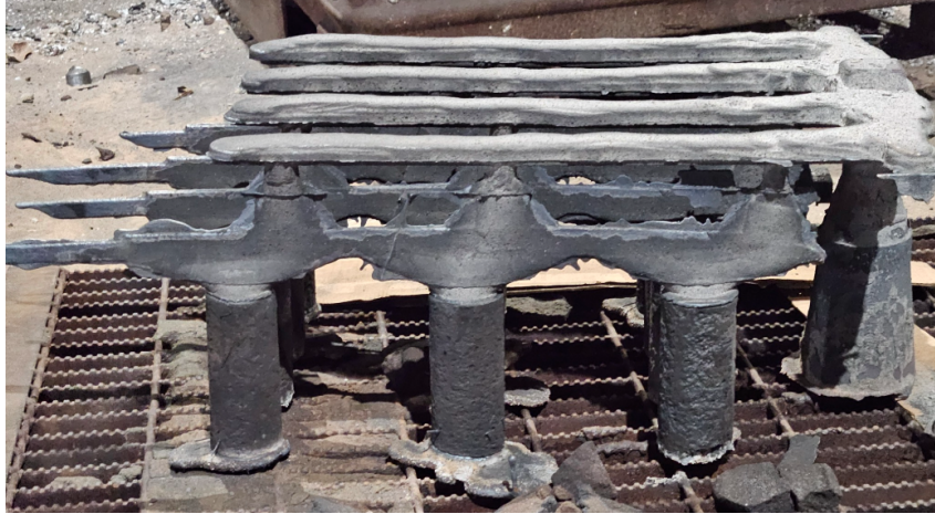
Figure 2) Solidification model using FLOW-3D to ensure the pour cup, gates, and risers will solidify after the swords. This minimizes shrinking and unwanted materials in the swords. a) shows the initial pour, b) shows the metal cooling in the risers and pour cup after 42 seconds, c) simulated porosity results after solidification, and d) the results of the pour after shaking down the mold.
