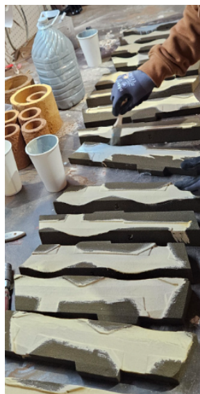
Figure 3) Applying Zircon wash to cores for smooth surfacing from sand mold.
