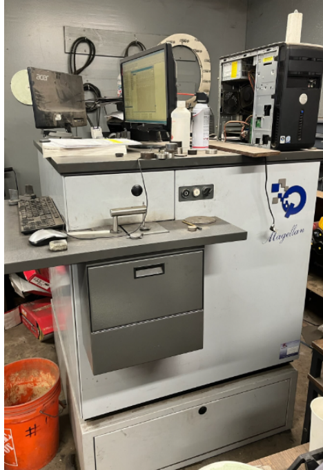
Figure 6) Optical emission spectrometer used to determine composition of a sample of the molten steel alloy prior to casting.
