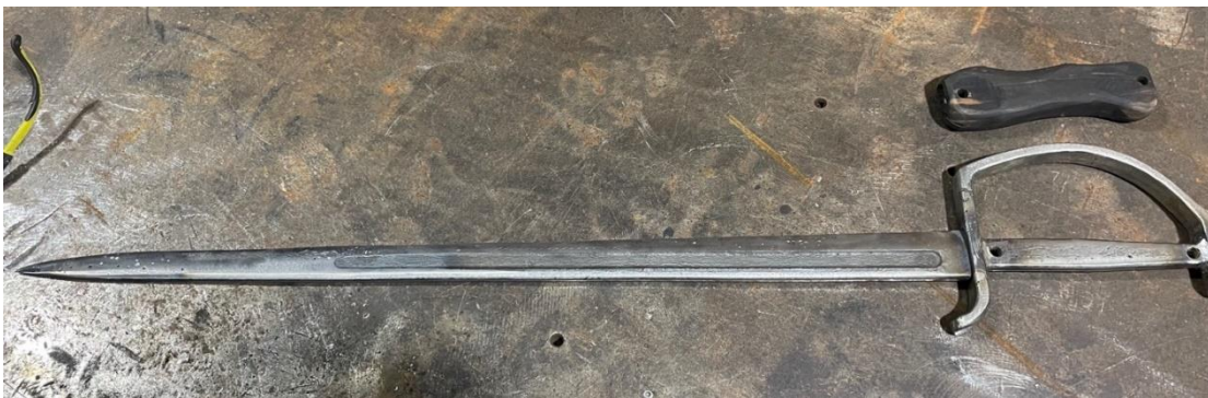
Figure 12: Full view of partially grinded sword alongside handle, unassembled
