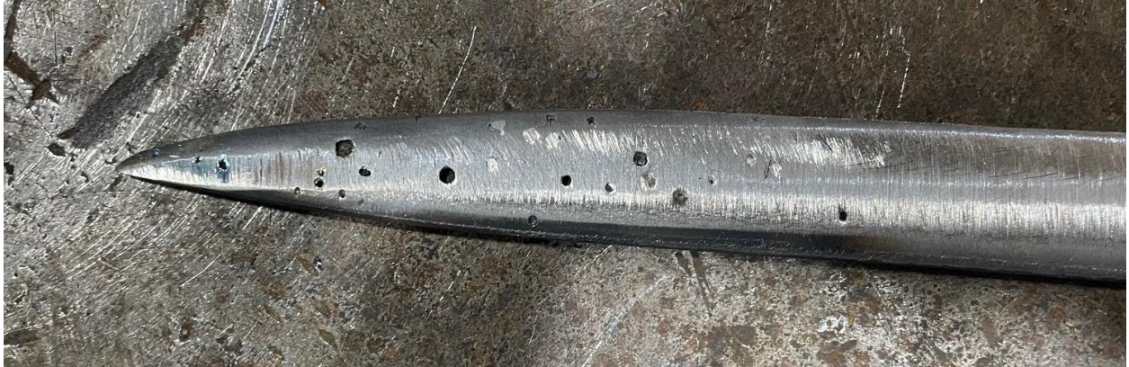
Figure 13: Pitting exhibited on blade tip during post process
