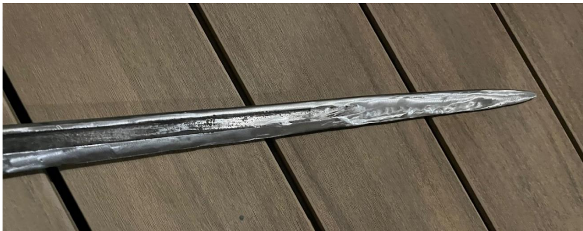
Figure 15: End of the blade, view of material distortion
