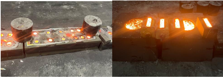
Figure 2 and 9: Gating after Pour: Sword and Guard
