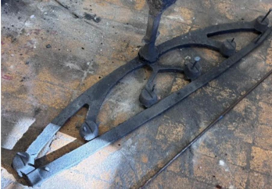
Figure 12. The final casting after an hour of cooling and the mold was shaken out
