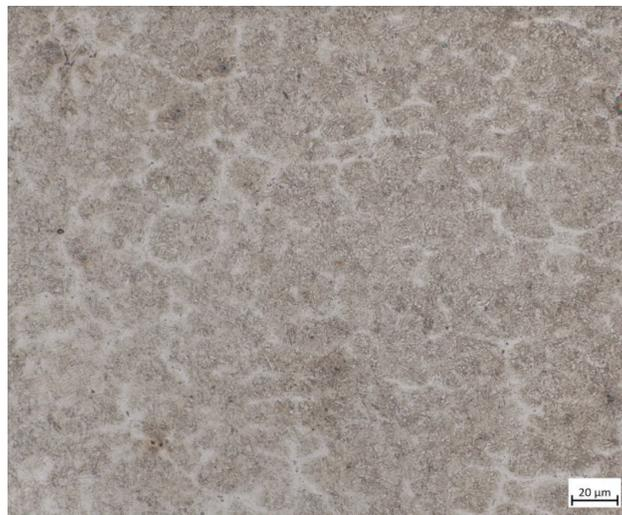
Figure 14. Microstructure of quenched sword showing fine lath martensite
