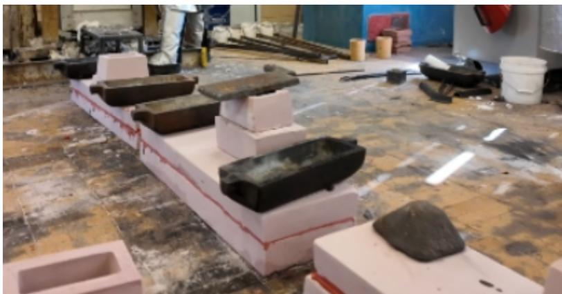
Figure 10. The assembled mold lined up next to the induction furnace, ready for casting
