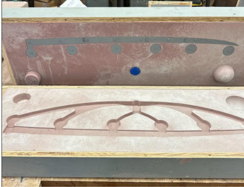
Figure 9. The mold curing in the flask before being removed and assembled with the pattern indentation
