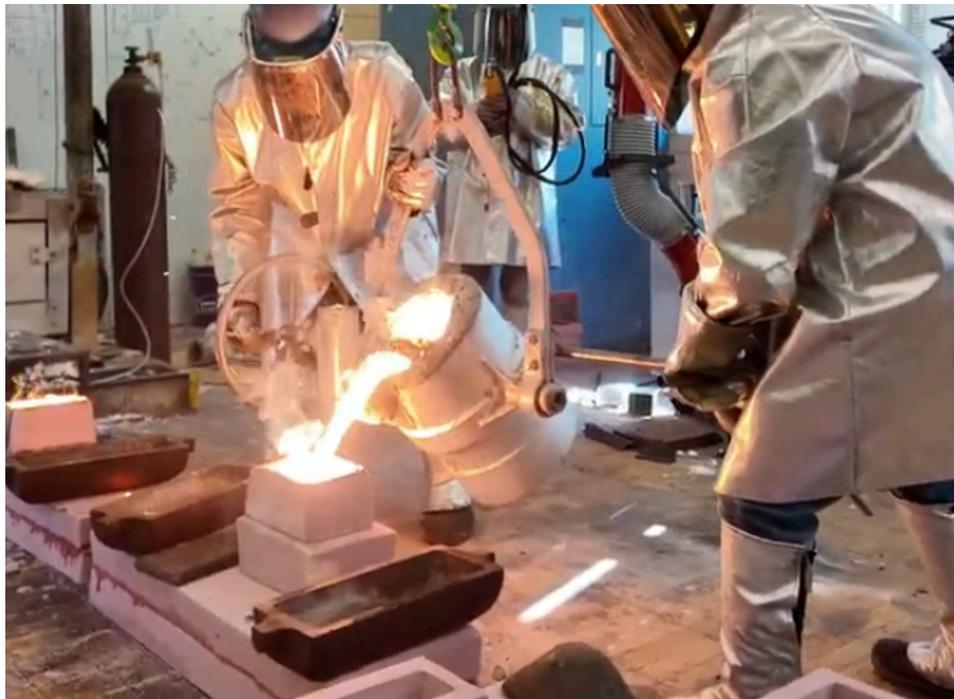
Figure 11. The liquid metal being poured into the assembled mold
