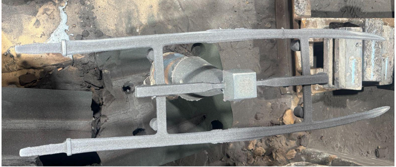
Figure 14. Sword replica raw casting (cast and photographed by Temperform).
