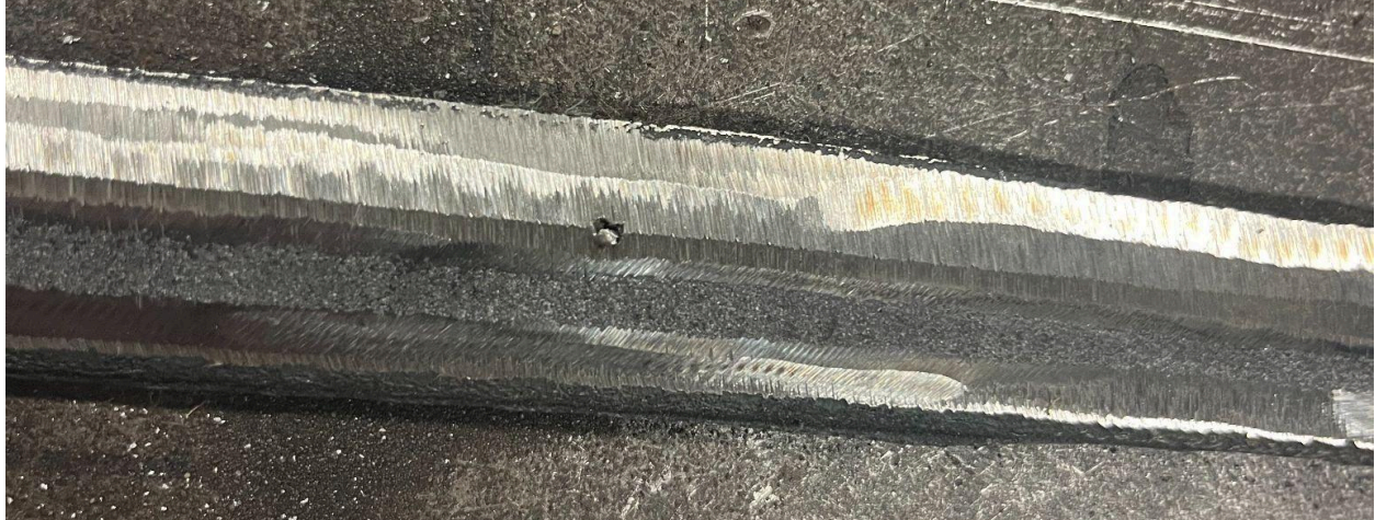
Figure 16. Porosity defect exposed while grinding the sword replica's edge.
