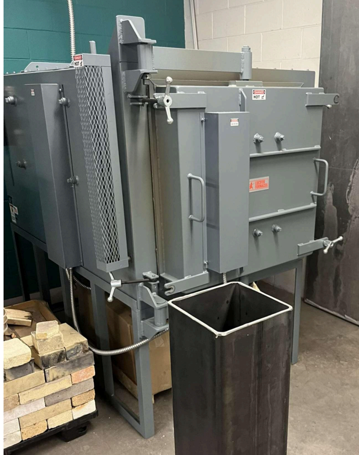
Figure 15. MTU's Lucifer Furnaces brand furnace and the oil quench used for the quench and temper heat treatment.
