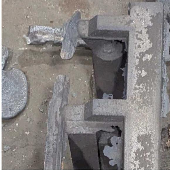
Figure 7: Tip misrun in first batch of as-cast blades.
