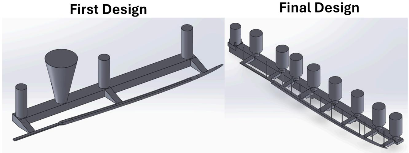
Figure 6: Horizontal casting design. First iteration (left) and final iteration (right) of horizontal design.
