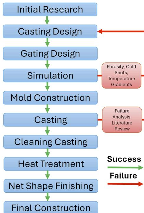
Figure 1: SFSA Cast in Steel flow chart of competition milestones.
