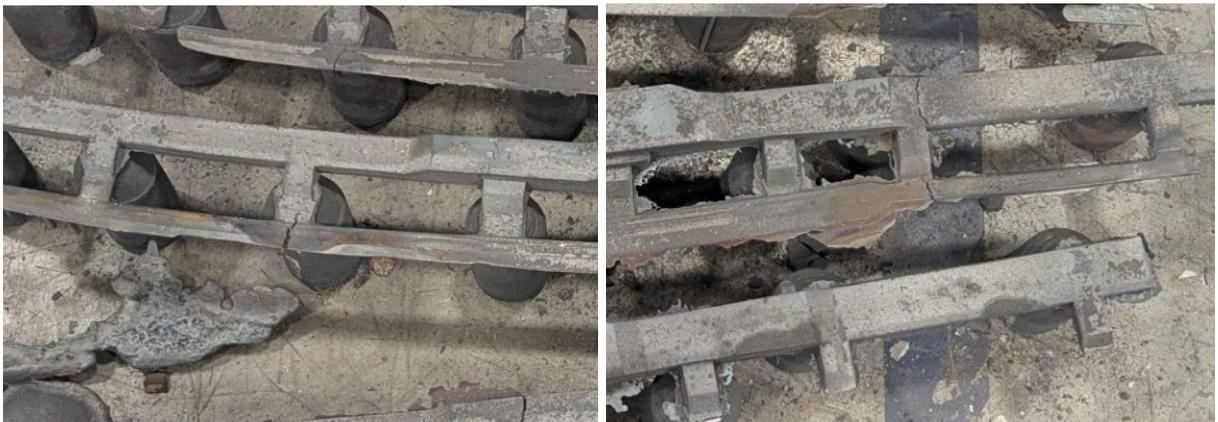
Figure 8: Stress fractures along the blade width. One is seen near the tip and the other at the base of the tang.
