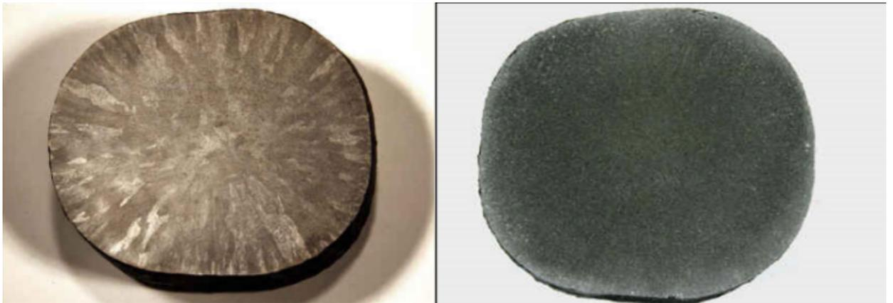
Figure 2: Cast steel showing a solidification microstructure (left) and normalized steel(right)
