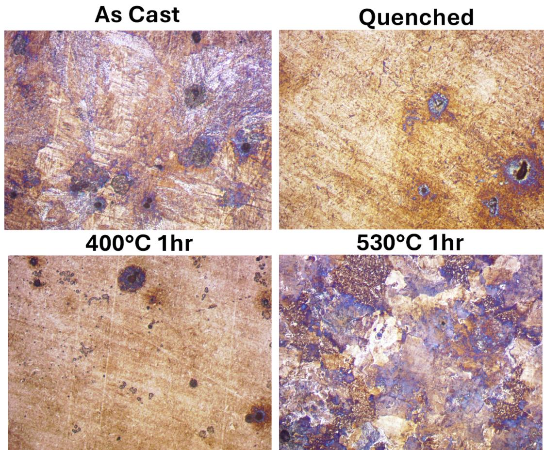
Figure 10: Etched micrographs of 9260 steel at different temperings. All at 20x magnification.
