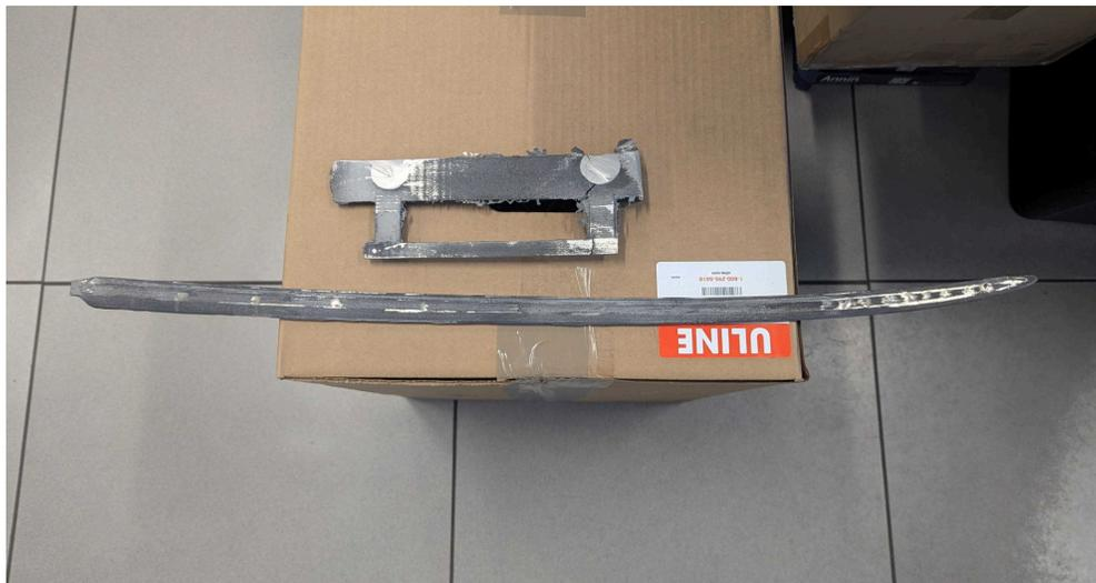
Figure 9: Final sword casting, showing a detachment from the tang due to cracking from runner solidification.
