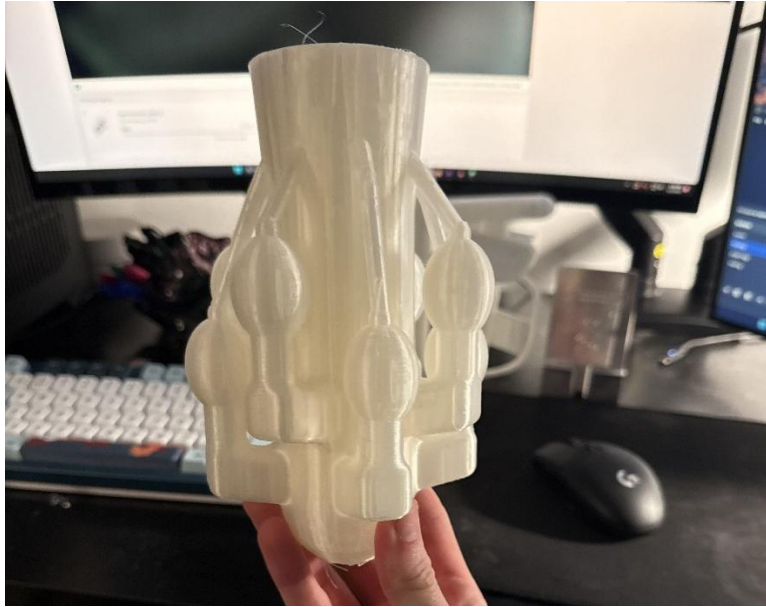
Figure 10: Pommel tree pattern 3D printed with Polycast filament.
