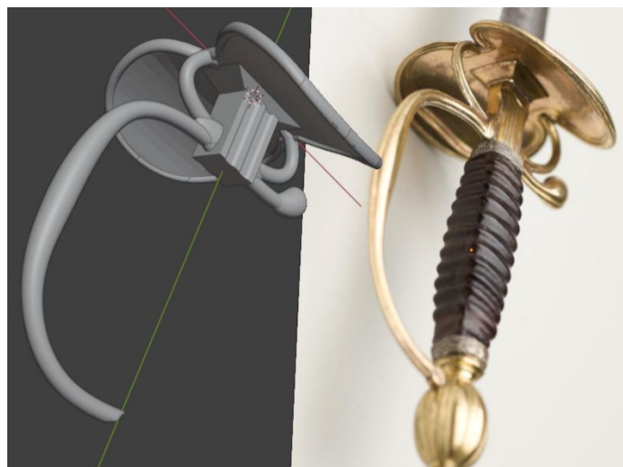
Figure 8: Hilt CAD model with reference photo.
