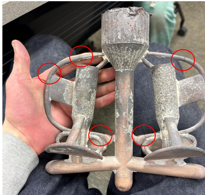
Figure 13: Hilt casting, the red circles indicate hot tear locations.
