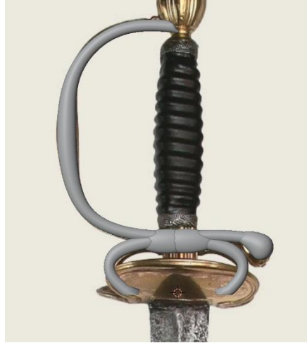
Figure 4: Knuckle guard CAD model with reference picture.
