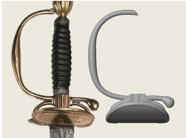
Figure 7: Hilt CAD model with reference photo.
