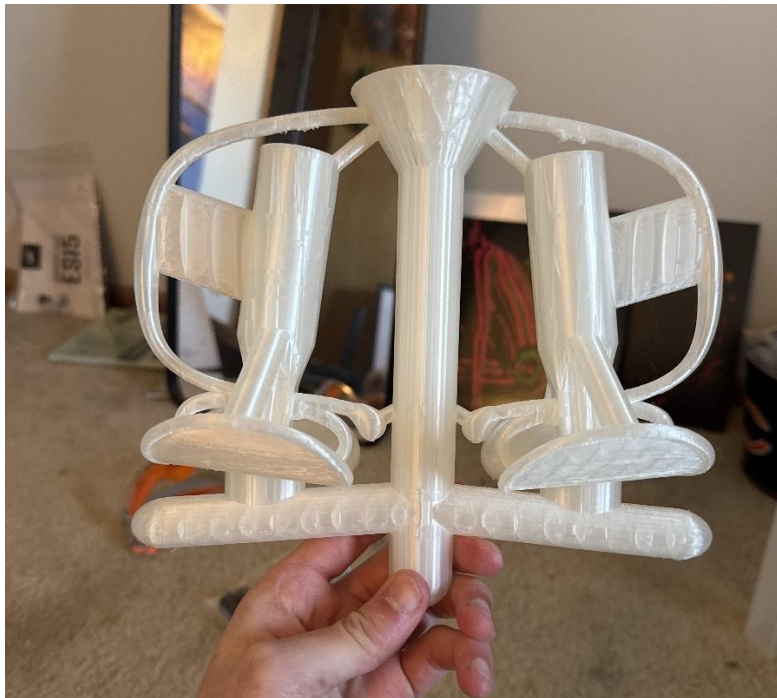
Figure 11: Hilt tree pattern 3D printed with Polycast filament.
