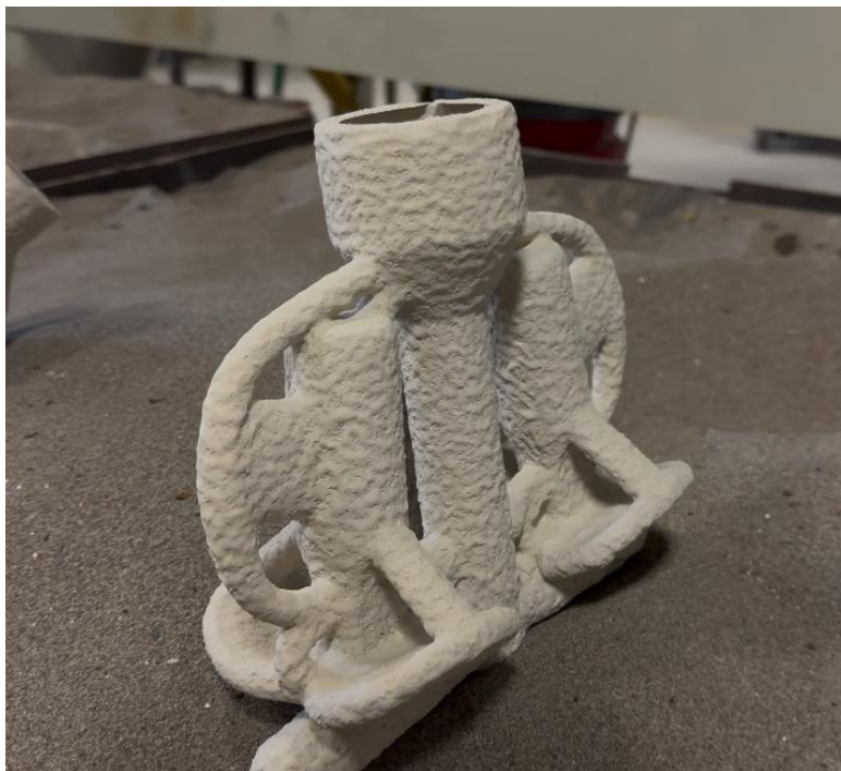
Figure 12: Final hilt shell before casting.
