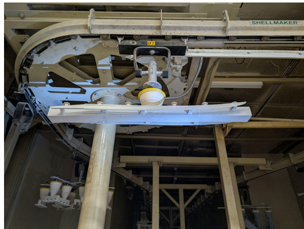
Figure 3: Gating system with first coat of slurry.
