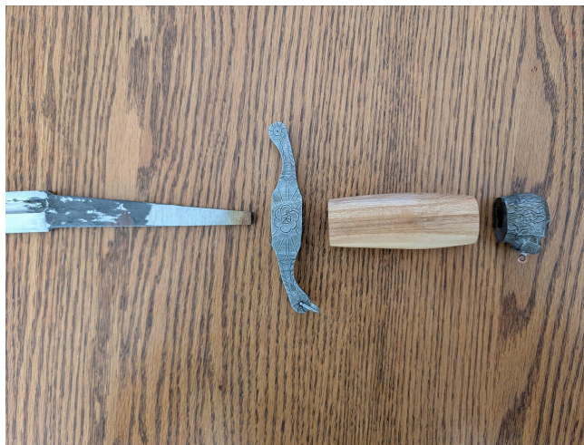
Figure 5: Tang extends through all handle components. Figure 6: The completed handle.
