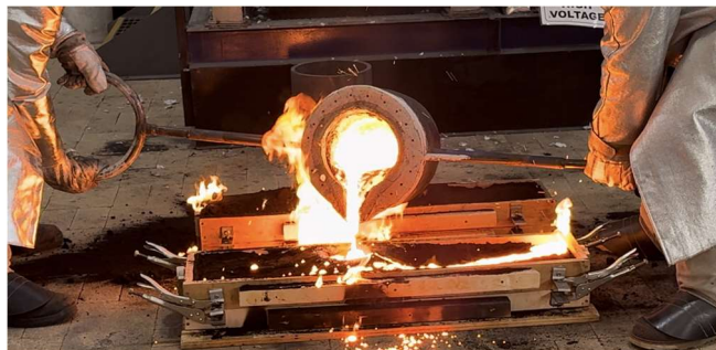
Figure 26 - Iteration 2 Flasks Catching Fire
