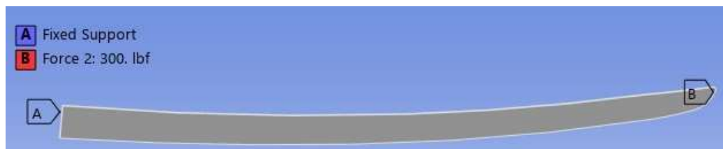
Figure 11 – Parameters for Slashing on the Edge
