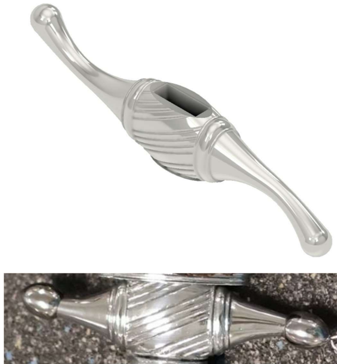
Figure 7 - Guard CAD (Top) and Guard Final (Bottom)
