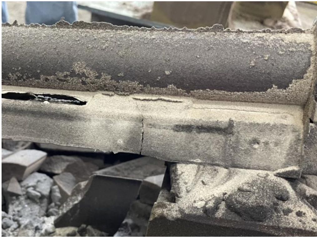
Figure 4.5: On the mold that wasn't dumped, the riser contraction led to bending stress in the blade, causing a crack a few inches from the handle.
