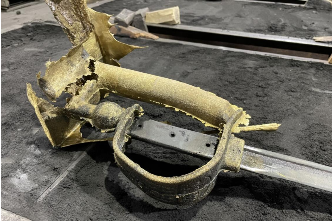
Figure 4.9: As-cast hilt, broken out quickly and quenched to minimize changes to blade metallurgy.
