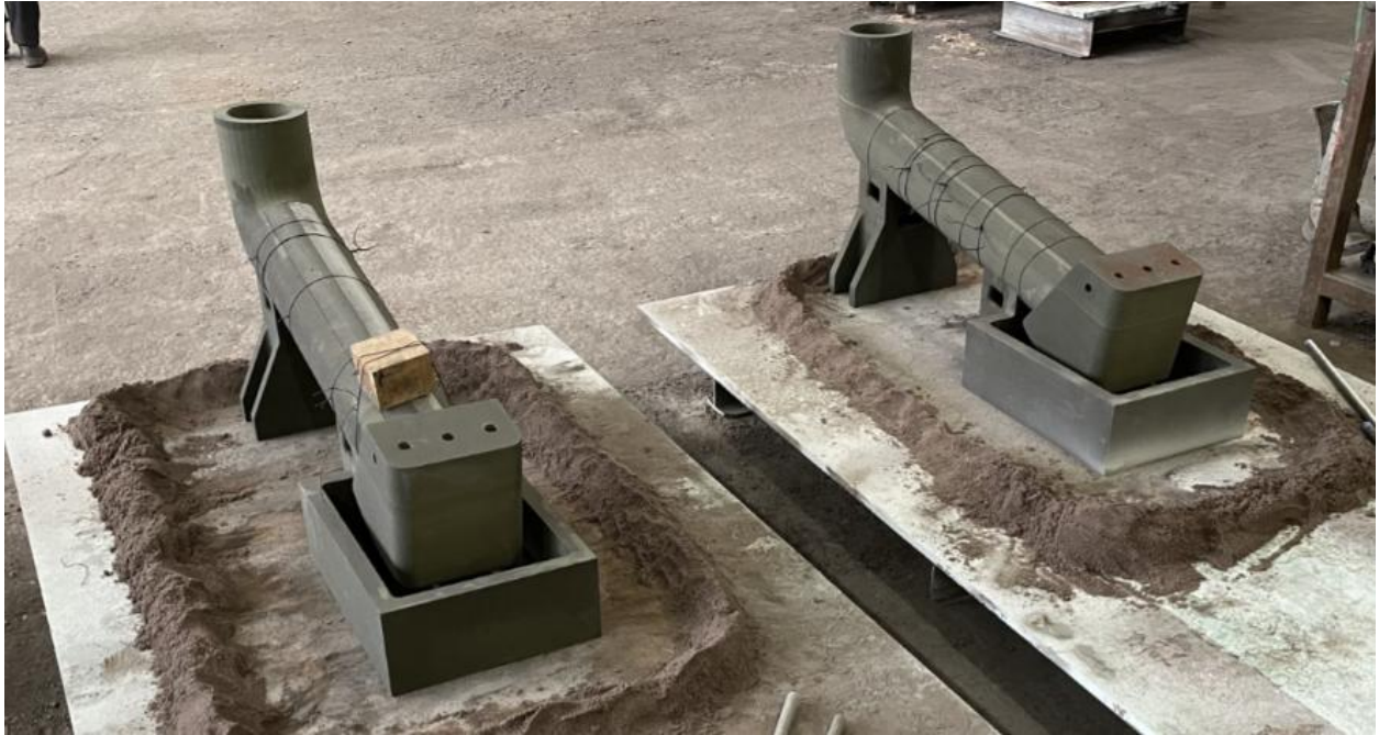
Figure 4.2: Assembled blade molds, enough to pour six blades.
