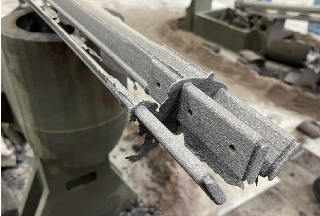
Figure 4.4: Three intact, straight blades requiring minimal grinding work from the mold that was dumped successfully.
