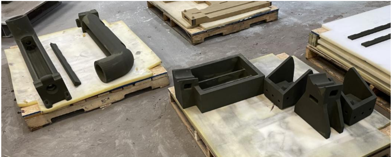
Figure 4.1: 3D sand printed blade mold parts before assembly.
