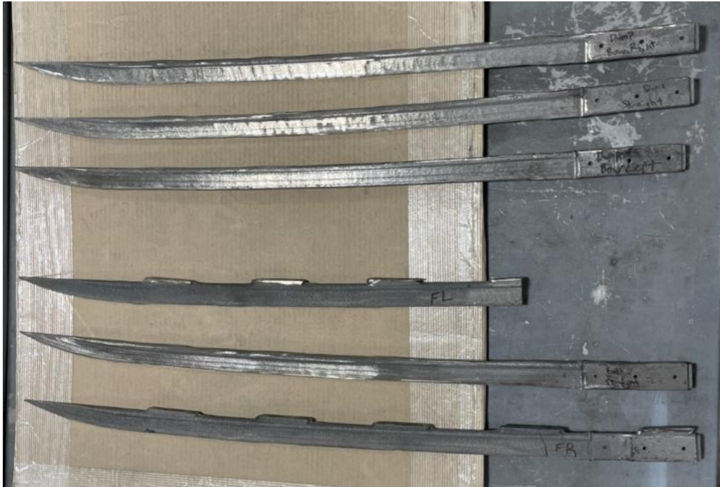
Figure 4.6: Blades during initial grinding to remove the remaining riser and gating material. On the top, three blades from the dumped mold. On the bottom, the blades from the mold that had not been dumped.
