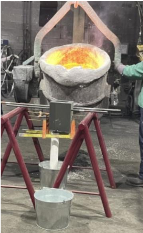
Figure 4.8: Bronze about to be poured into the hilt mold.
