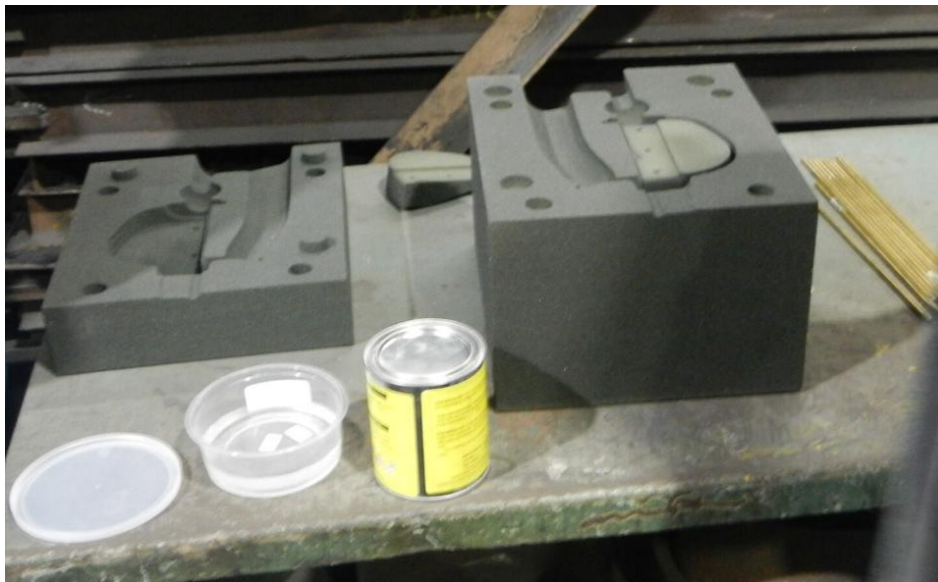
Figure 3.5: Assembly of hilt mold showing internal cavity and cores.
