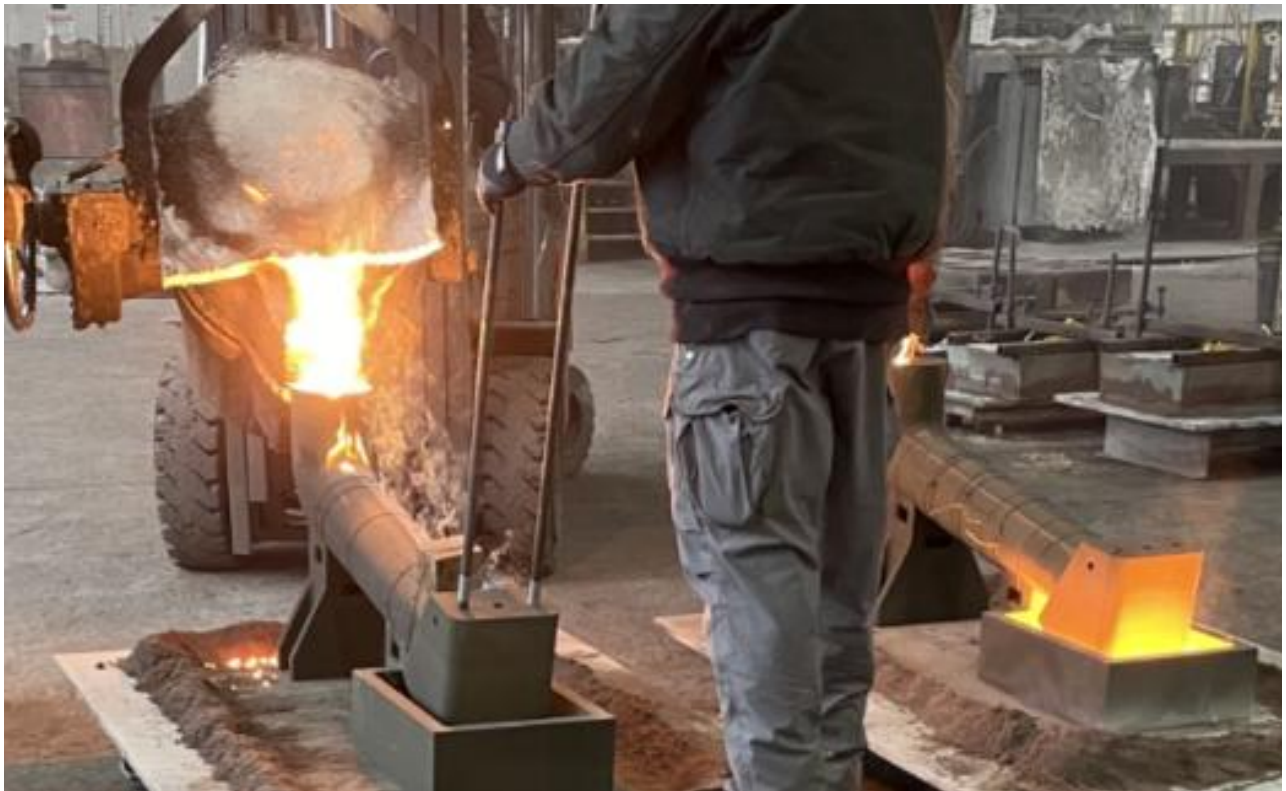
Figure 4.3: On the right, the mold has been successfully dumped into ingots with the sand valve. The second mold is being poured on the left and will not be dumped.
