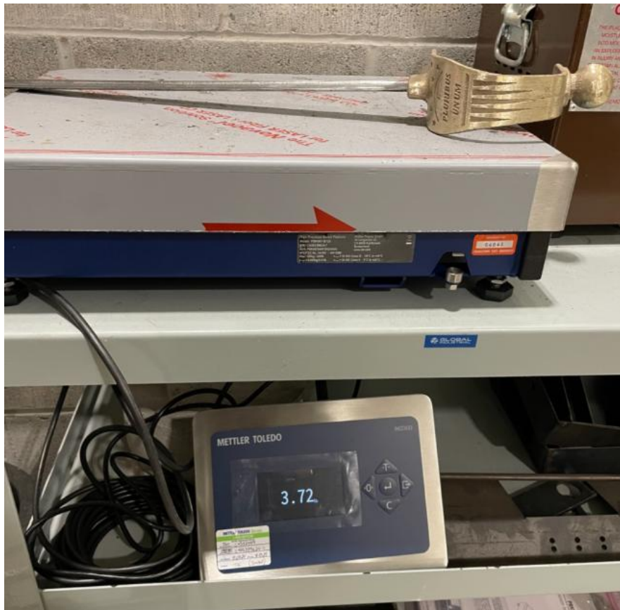
Figure 5.2: Weighing the final blade. (Recorded as 3.8 lbs. to consider any small additions to the grip)
