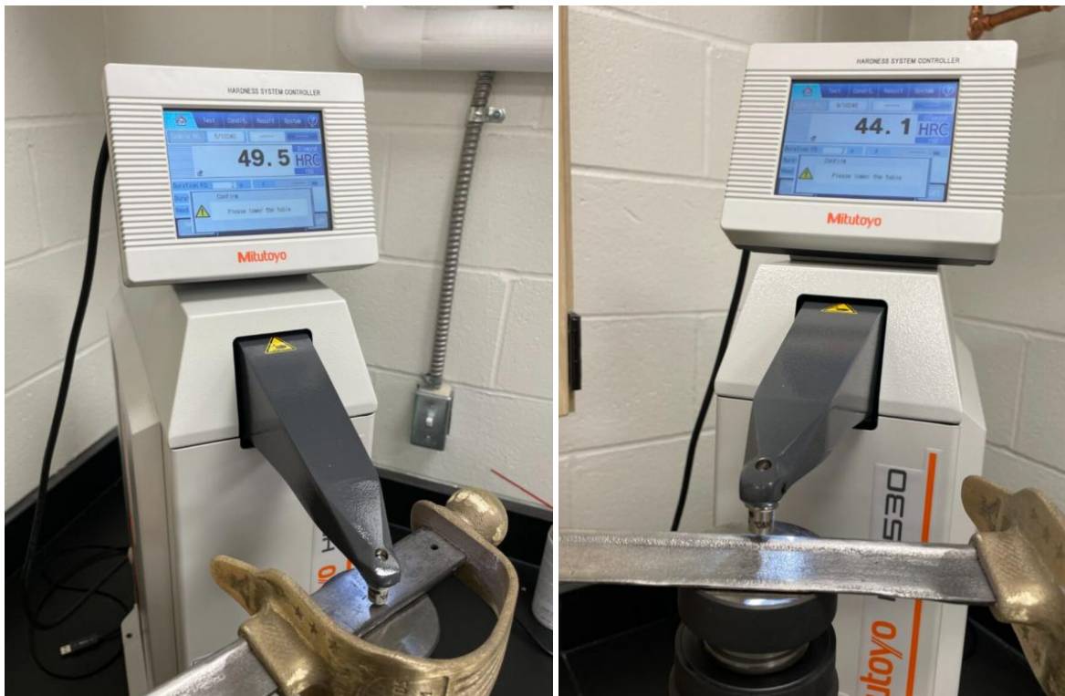
Figure 5.3: Rockwell Hardness Tester used to measure the final hardness of the handle and blade spine on the submitted sword. The result indicates the intended heat treatment was completed.
