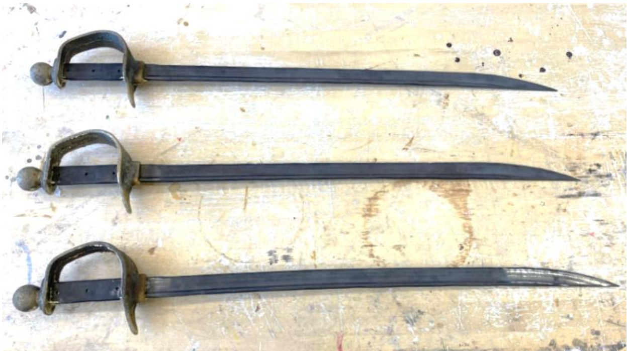
Figure 4.10: Swords with all risers ground off, ready for details, polishing, and sharpening.
