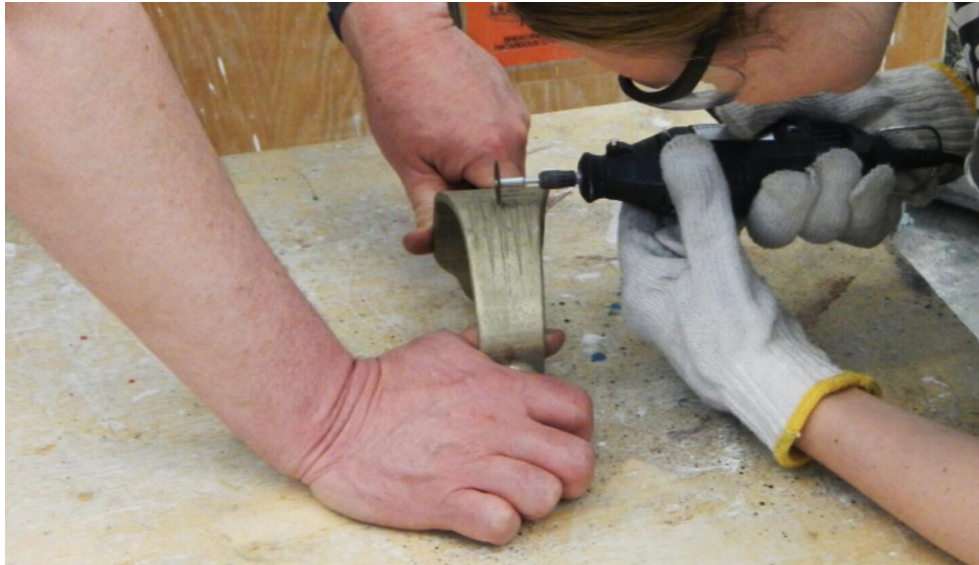
Figure 4.11: Removing flashing and cleaning out details on the hilt.
