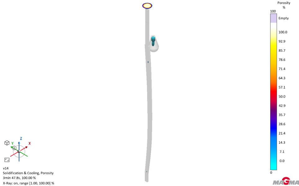
Figure 5: Porosity Percentage in the Results Perspective of MAGMAsoft
