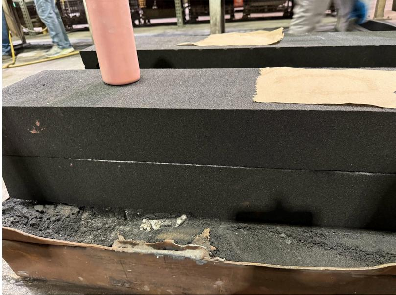
**Figure 21:** Cope and drag assembly
