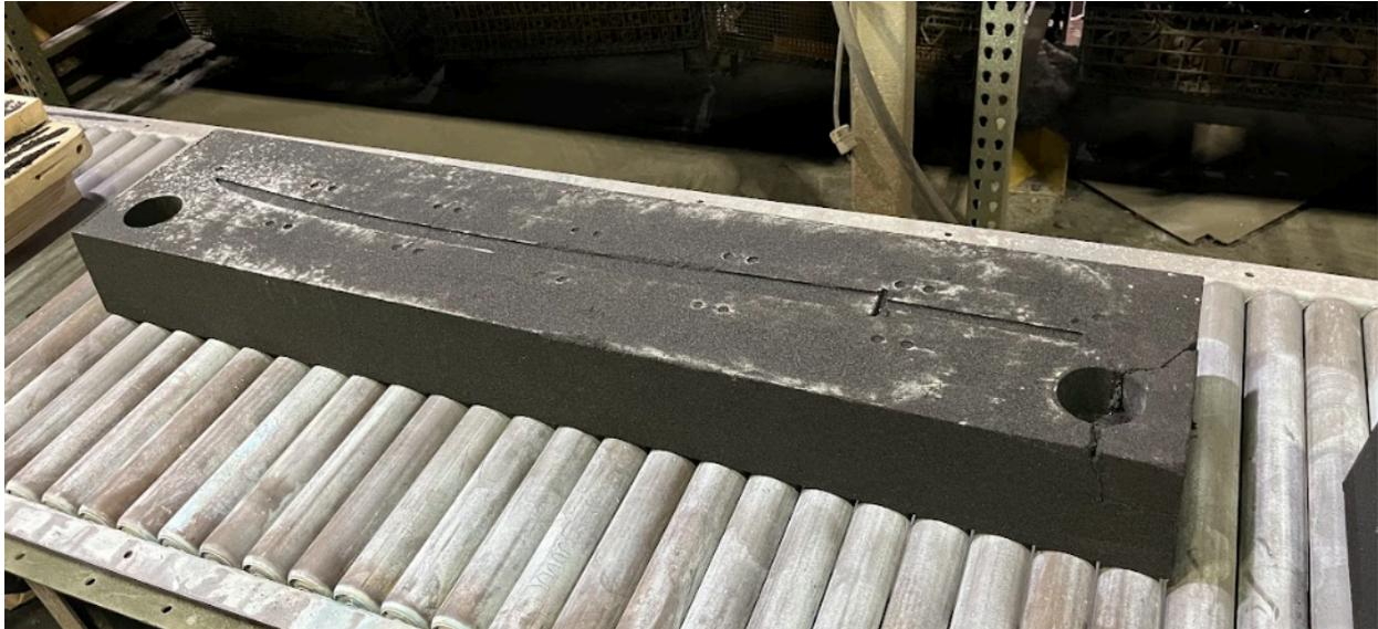
**Figure 18:** Finished and released drag mold.
