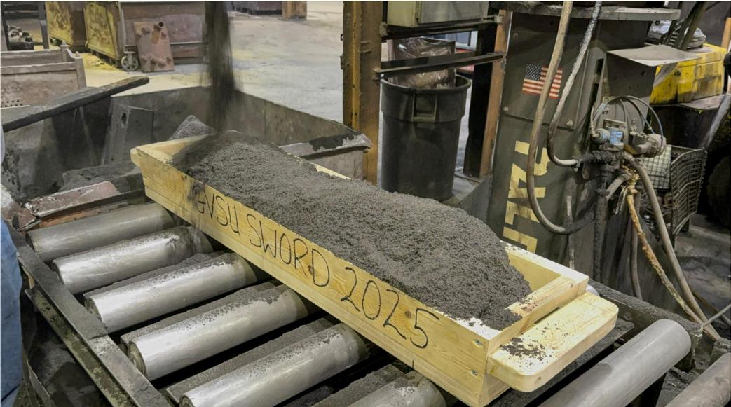
**Figure 16:** Airset sand being poured into the mold.
