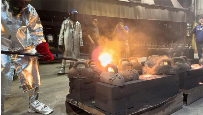
**Figure 23:** Metal being cast into the molds.
