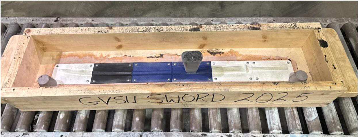
**Figure 9:** 3D printed pattern pieces placed and fastened in the cope flask.
