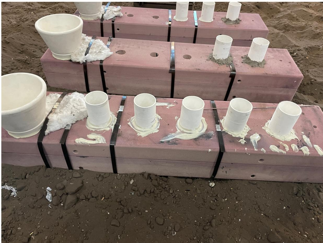
Figure 7: Mold Condition Before Pouring
