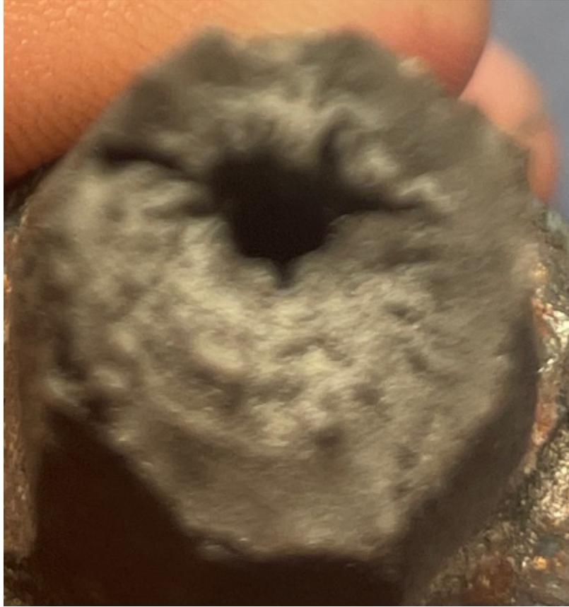
*Figure 18: As-Forged Test Bar Fracture Surface*
