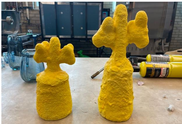
Figure 8: Investment Molds Prior to Burn-out and Firing
