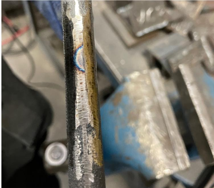
*Figure 10: Weld Repair*
