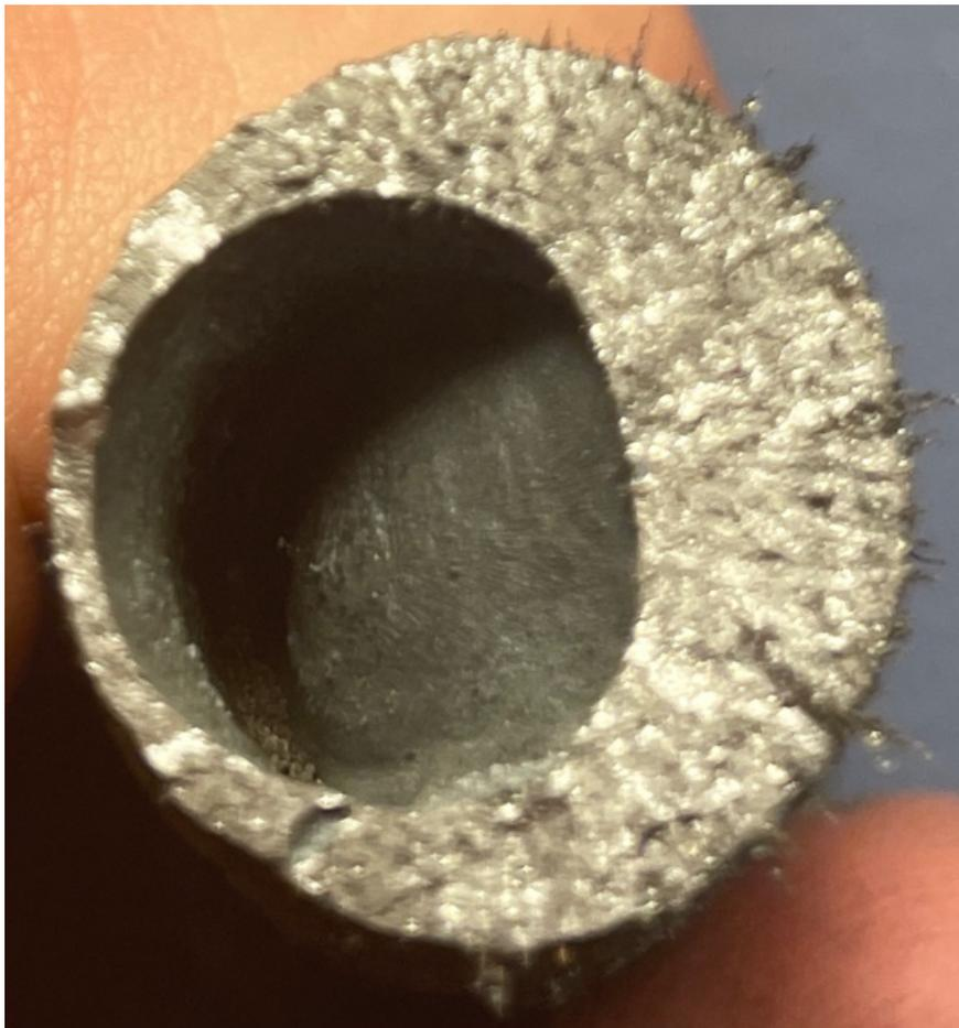
*Figure 17: As-Cast Test Bar Fracture Surface*
