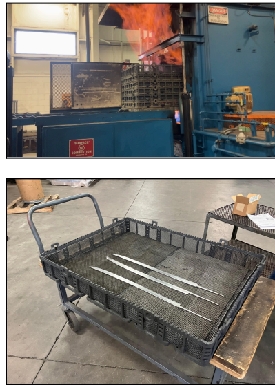
Figure 18: Blades entering heat treat
