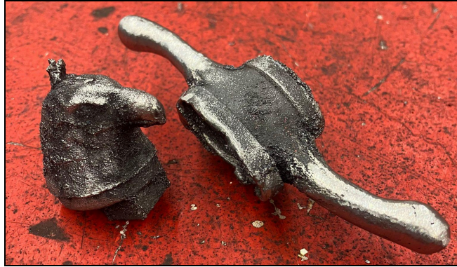
Figure 30: Final Guard and Pommel Cast (Guard partially ground)
