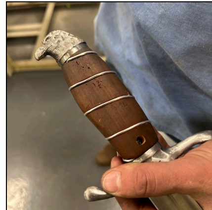
Figure 39: \frac{1}{4} in Hole For Epoxy Pour 2
