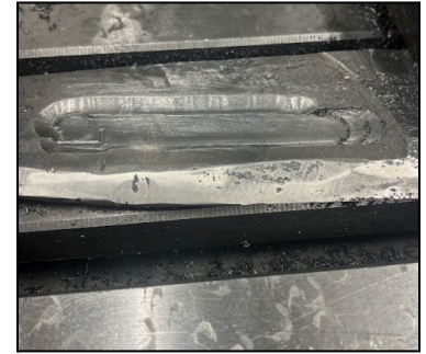
Figure 13: Milling the fuller
