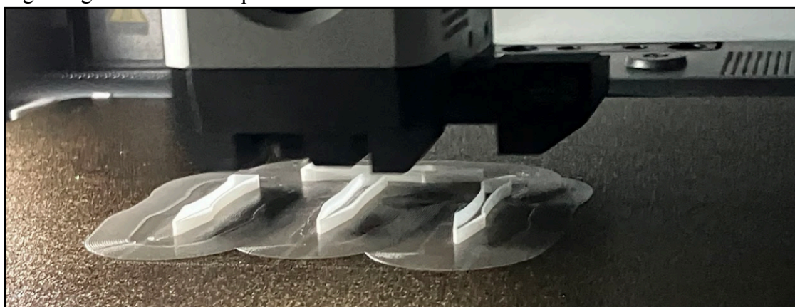
Figure 5: Initial 3D print of blade sections
