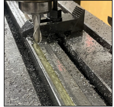
Figure 16: End milling the fuller
